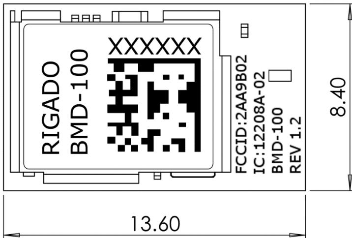
Figure 6 – Module Marking – Rev A
