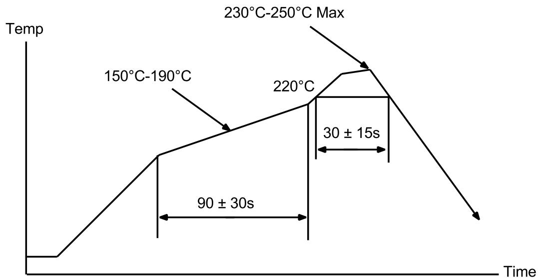
Figure 8 - Reflow Profile for Lead Free Solder
