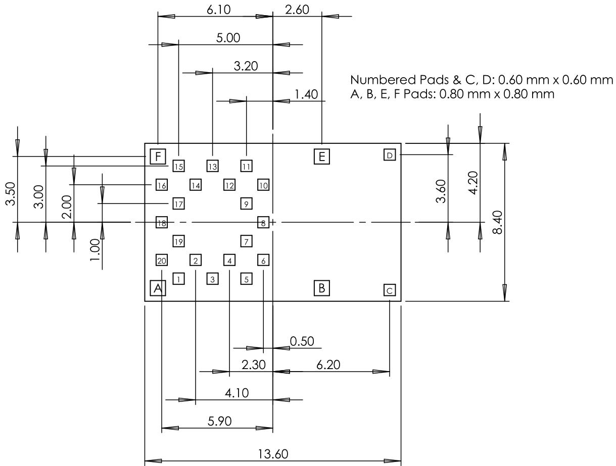
Figure 5- Module Dimensions
