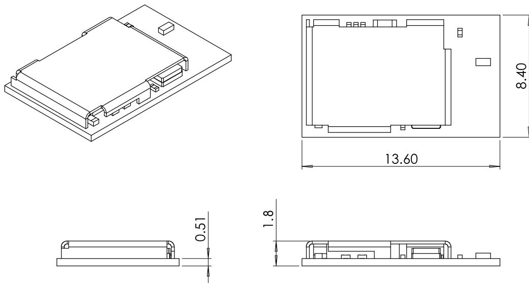
Figure 4- Module Dimensions
