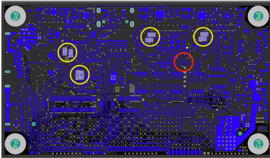
If the resistors are removed and there is no CSI-2 module connected then the high voltage will be 1.8V on the 3.3V side. The B10x have 10kOhm I2C pull up resistors on the module. If a module w/o I2C pull up resistors is connected, then 10kOhm pull up resistors should be added on the J100. The picture below shows how the B10x modules are connected. Please check the I2C section for details. Top: B101 (2 lanes). Bottom: B102 (4 lanes).
