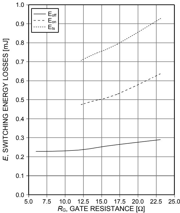
Figure 13. **Typical switching energy losses as a function of gate resistance**
