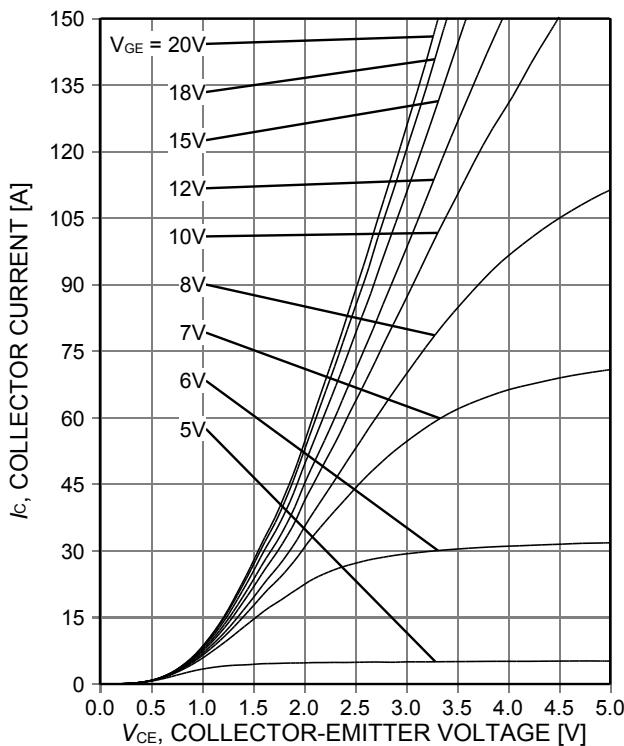
**Figure 5. Typical output characteristic**
