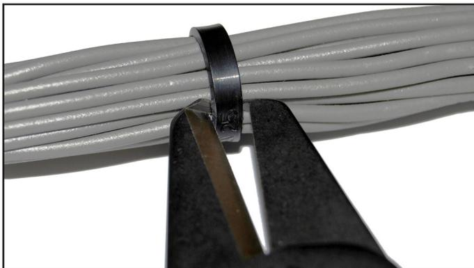
Now you can quickly remove cable ties without damaging the wire harness. The safety guards on the tip of the MG-1300 cable tie removal tool slides behind the cable tie strap to prevent the sharp blades from contacting and damaging the bundled items. The ergonomic, cushion grip handles and scissor action produce a clean cut.
