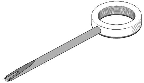
This Insertion tool is used for insertion of .062" diameter series pin and socket male and female terminals in plug and receptacle housings. This tool is designed to assure proper seating of terminals and reduce operator fatigue.
