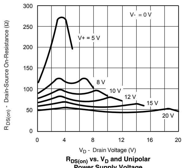
**$R_{DS(on)}$  vs.  $V_D$  and Unipolar Power Supply Voltage**
