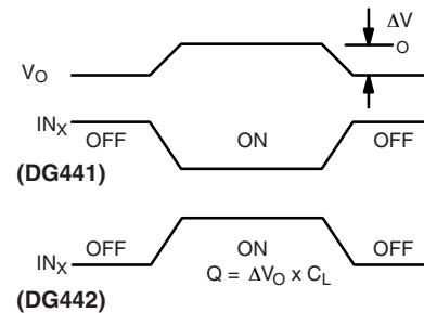
**Figure 3. Charge Injection**
