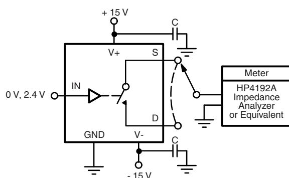
**Figure 6. Source/Drain Capacitances**
