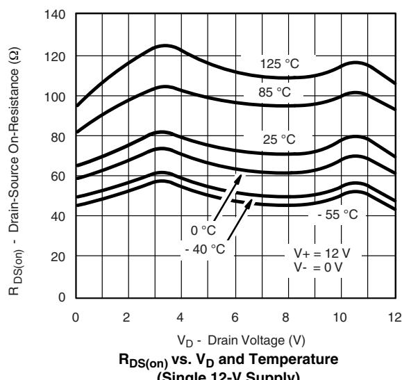
**$R_{DS(on)}$  vs.  $V_D$  and Temperature
