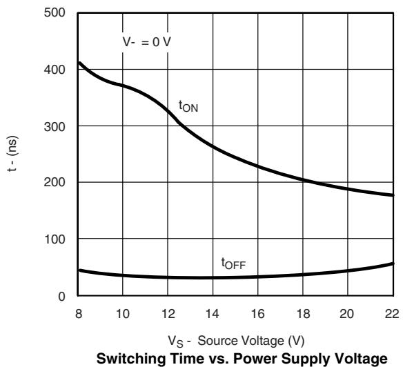
Switching Time vs. Power Supply Voltage
