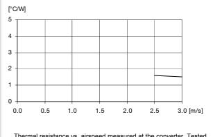
Thermal resistance vs. airspeed measured at the converter. Tested in wind tunnel with airflow and test conditions as per the Thermal consideration section.  $V_I = 27 \text{ V}$ .
