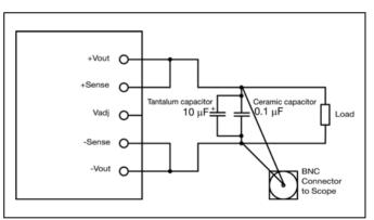
Output ripple and noise test setup
