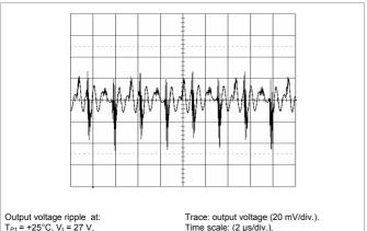
Output voltage ripple at:  $T_{P1} = +25$ °C,  $V_{I} = 27$  V, I<sub>O</sub> = 14.3 A resistive load. Trace: output voltage (20 mV/div.). Time scale: (2  $\mu$ s/div.).
