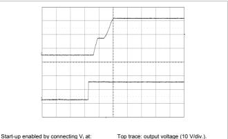
$T_{P1} = +25^{\circ}C$ ,  $V_{I} = 27$  V,  $I_{O} = 14.3$  A resistive load.
