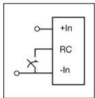
The products are fitted with a remote control function referenced to the primary negative input connection (- In), with negative and positive logic options available. The RC function allows the converter to be turned on/off by an external device like a semiconductor or mechanical switch.
