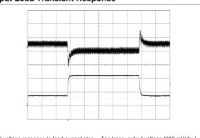
Output voltage response to load current stepchange (3.58-10.72-3.58 A) at: T<sub>P1</sub> = +25°C, V<sub>1</sub> = 27 V. Top trace: output voltage (200 mV/div.). Time scale: (0.1 ms/div.).
