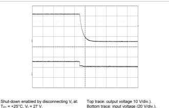
$T_{P1} = +25^{\circ}C$ ,  $V_1 = 27$  V,  $I_0 = 14.3$  A resistive load.
