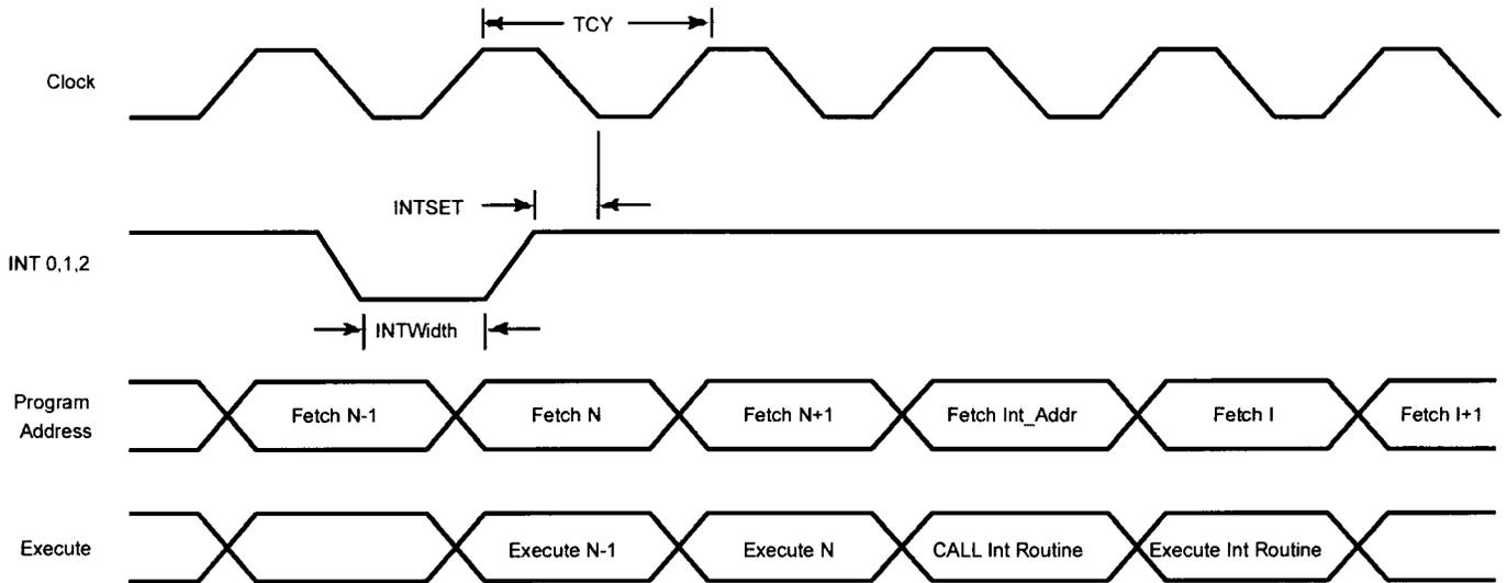
Figure 11. Interrupt Timing
