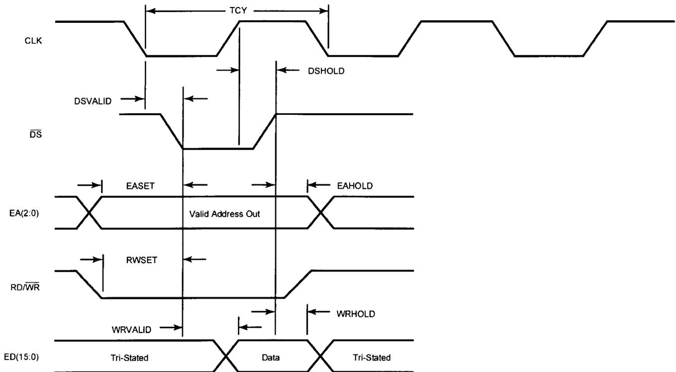
Figure 9. Write Timing
