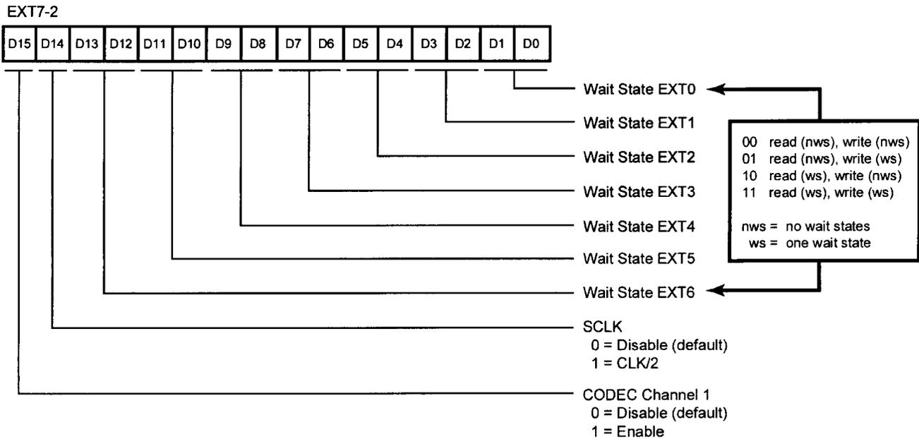
Figure 24. Wait-State Generator and CODEC Interface Control Register
