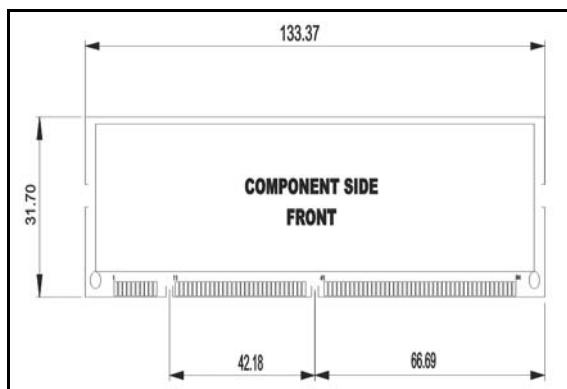
Figure 11: DIMM Dimensions
