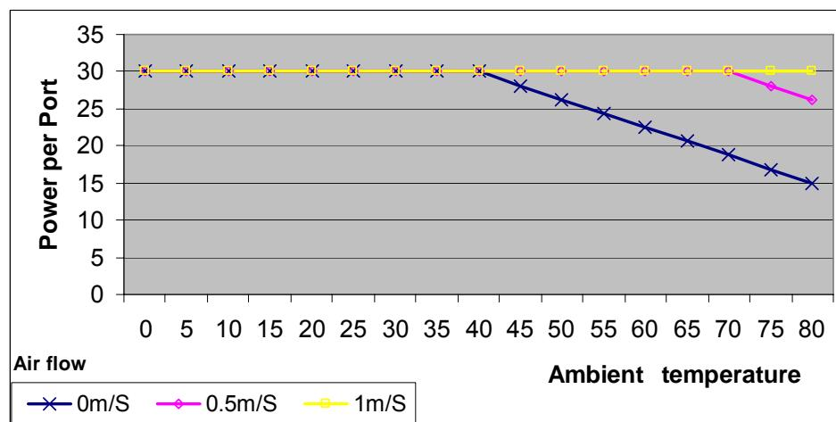
**Figure 3: Power per Port for two DIMMs (48 ports)**
