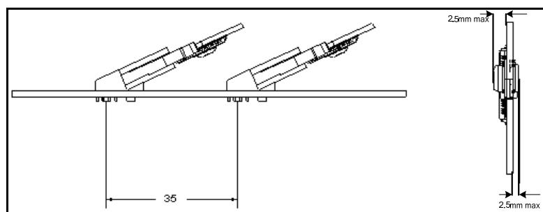
Figure 12: Mechanical Outline of the PD671xxx DIMM
