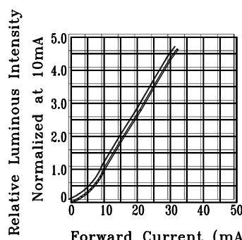
Fig.4 Relative Luminous Intensity
