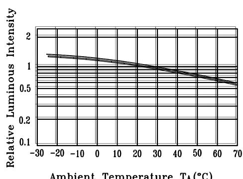
Fig.5 Luminous Intensity vs.
