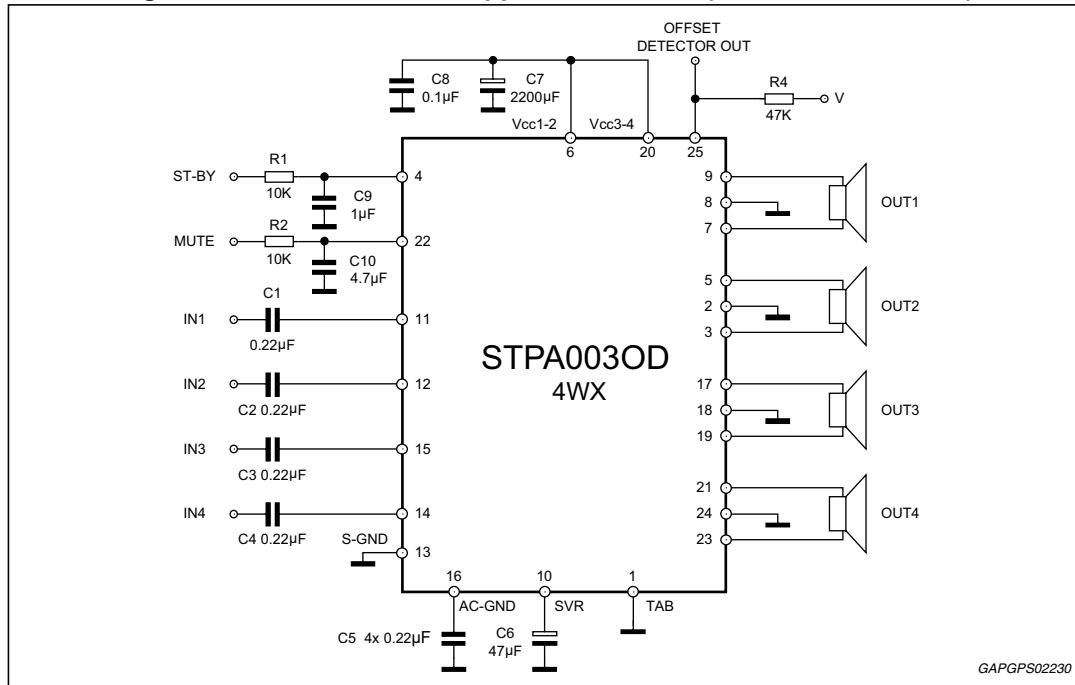
**Figure 3. Standard test and application circuit (Flexiwatt27 with CD)**
