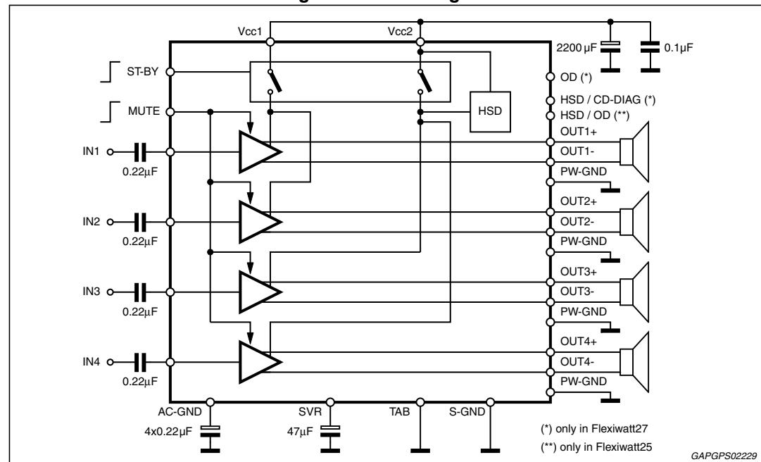
**Figure 2. Standard test and application circuit (Flexiwatt25 with OD)**
