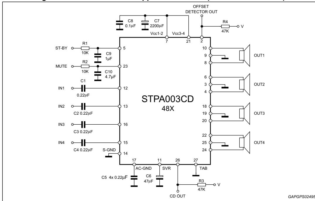
**Figure 4. Standard test and application circuit (Flexiwatt27 with HSD)**
