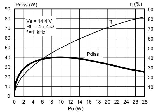
**Figure 18. Power dissipation vs. average output power (4 Ω, audio program simulation)**
