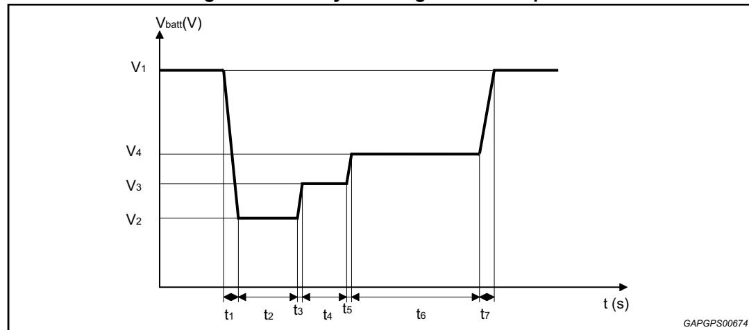
$V1 = 16 \text{ V}$ ;  $V2 = 6 \text{ V}$ ;  $V3 = 7 \text{ V}$ ;  $V4 = 8 \text{ V}$
