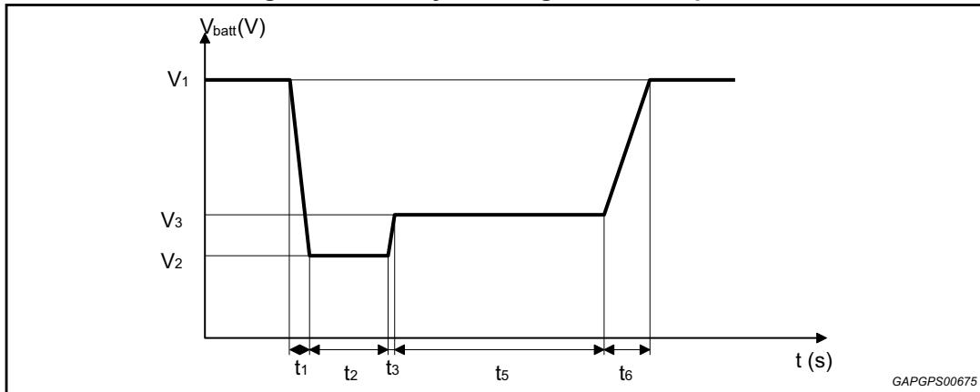
$V_1 = 16 \text{ V}$ ;  $V_2 = 6 \text{ V}$ ;  $V_3 = 7 \text{ V}$
