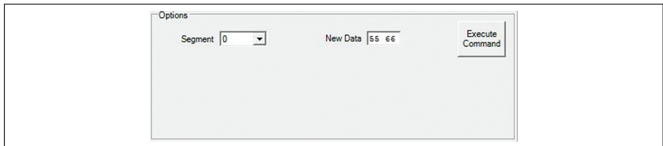
Figure 7. Write Memory Command Option for General-Purpose Writing
