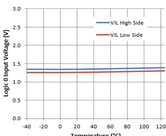
Figure 20. Logic 0 Input Voltage vs. Temperature
