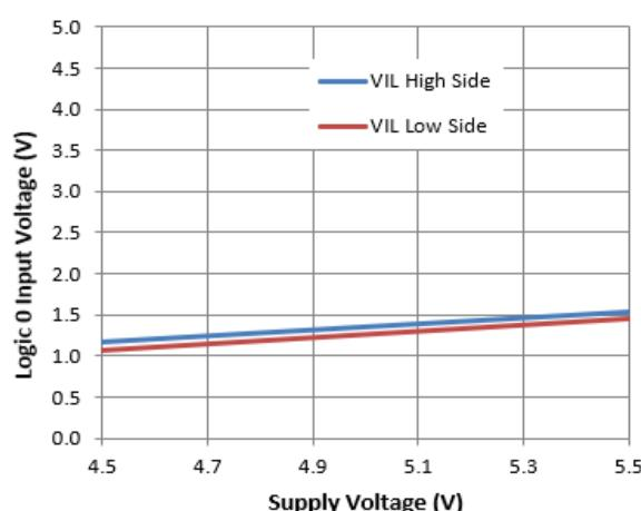
Figure 19. Logic 0 Input Voltage vs. Supply Voltage
