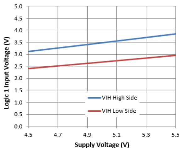
Figure 17. Logic 1 Input Voltage vs. Supply Voltage
