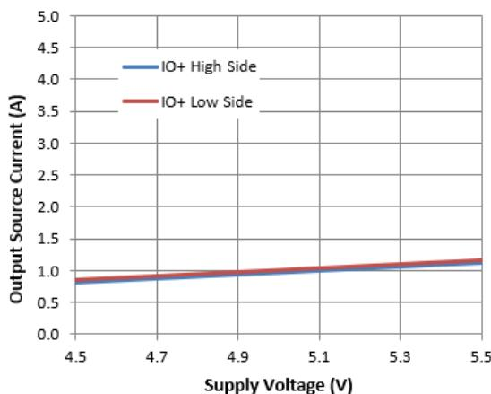
Figure 13. Output Source Current vs. Supply Voltage
