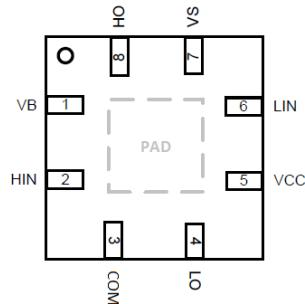
Top View: V-QFN3030-8 (Type TH)
