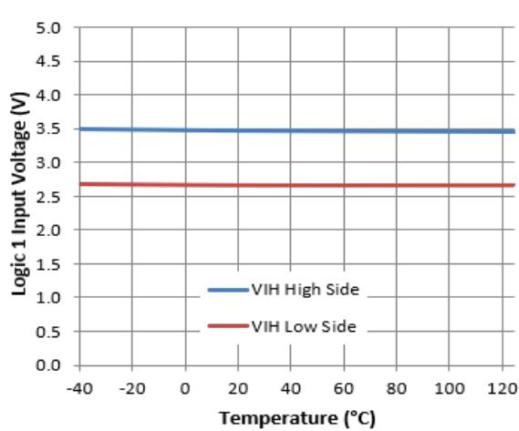
Figure 18. Logic 1 Input Voltage vs. Temperature
