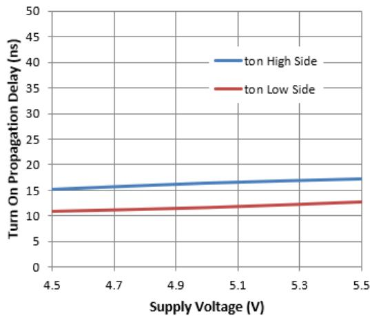
Figure 3. Turn-on Propagation Delay vs. Supply Voltage
