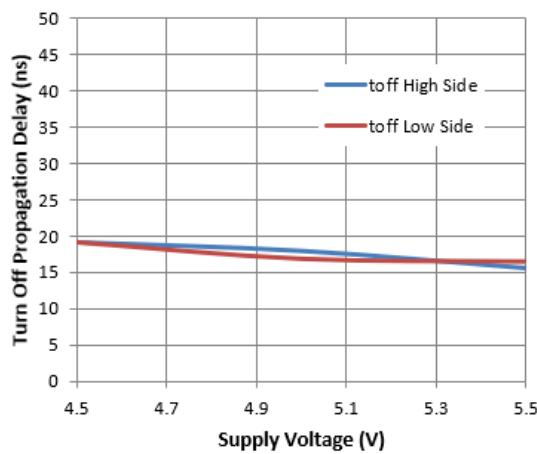
Figure 5. Turn-off Propagation Delay vs. Supply Voltage
