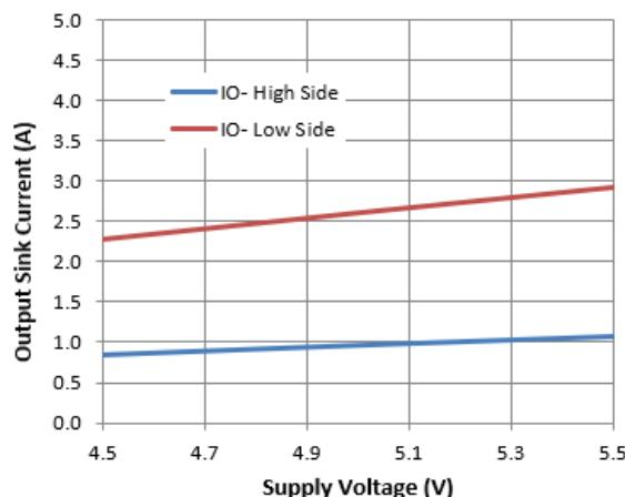
Figure 15. Output Sink Current vs. Supply Voltage
