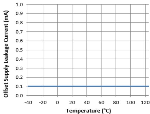
**Figure 21.** Offset Supply Leakage Current vs. Temperature
