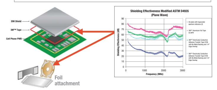
3M<sup>™</sup> Electrically Conductive Adhesive Transfer Tapes 9703, 9404, 9705, 9706, 9708, 9709, 9709S, 9709SL, 9712, 9713, 9714 and 7805 can provide FPC grounding and tapes 9708, 9709, 9709S, 9709SL and 7805 can increase the effective EMI Shielding through the bond line thickness leading to improved product EMI Shielding performance of the FPC.
