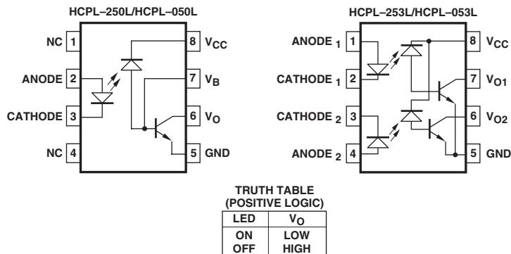
A 0.1  $\mu$ F bypass capacitor must be connected between pins 5 and 8.
