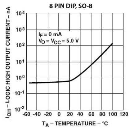
Figure 5. Logic high output current vs. temperature
