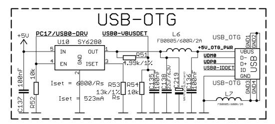
The USB\_OTG features Low Loss Power Distribution Switch SY6280 which protects the board in case the devices you have plugged to the USB\_OTG attempt to draw more current than 523mA combined. The maximum current available on the 5V USB\_OTG is exactly 523mA.
