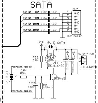
The SATA connector allows you to connect hard drives to the board. There is support for SATA drives in the official images. The connector is suitable for both regular hard-drives and SSD ones.
