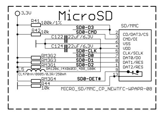
This slot is typically used for booting the OS, due to the larger capacities of the microSD cards (compared to SD or MMC cards). It is suggested to have an SD card with a proper Linux/Android image especially if you have ordered a version of the board without NAND memory. It is also recommended to use Class 10 (10MByte/sec) card for faster read/write operations, lower class cards (especially higher capacity ones) might slow down the whole system.
