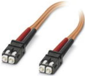
Assembled FO cable, zip cord cable, multi-mode fiberglass 50/125 µm, OM2, plug: SCRJ/SCRJ, degree of protection: IP20, for installation in cable ducts or control cabinets, length: 2 m
