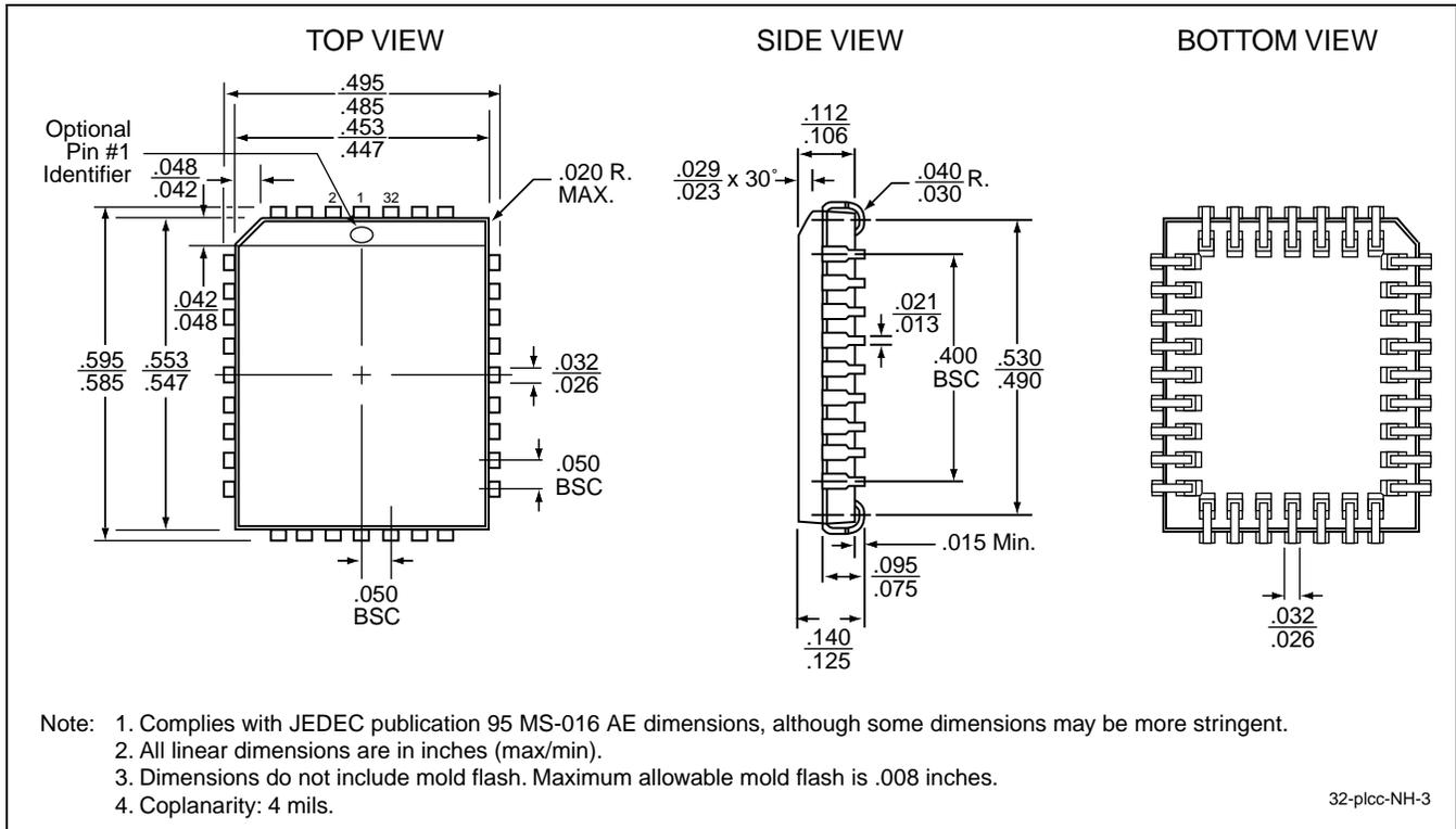
**FIGURE 17: 32-lead Plastic Lead Chip Carrier (PLCC)**
