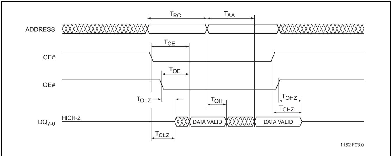
FIGURE 6: Read Cycle Timing Diagram for GLS27SF512/010/020
