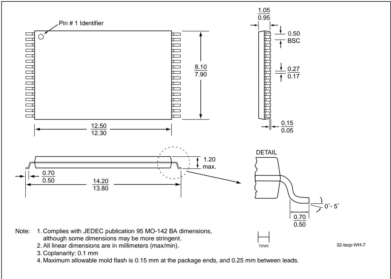
**FIGURE 18: 32-lead Thin Small Outline Package (TSOP) 8mm x 14mm
