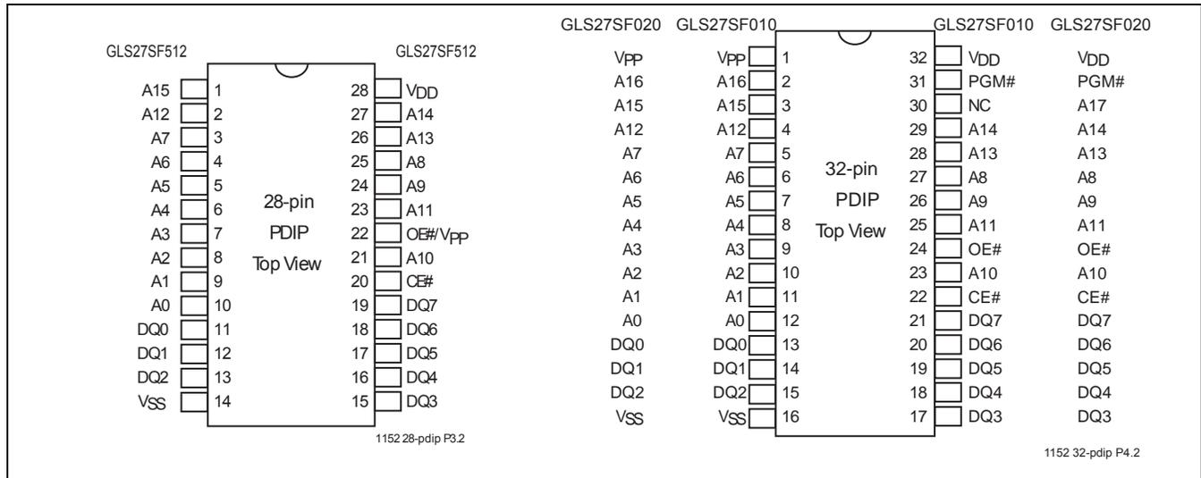
FIGURE 5: Pin Assignments for 28-pin and 32-pin PDIP
