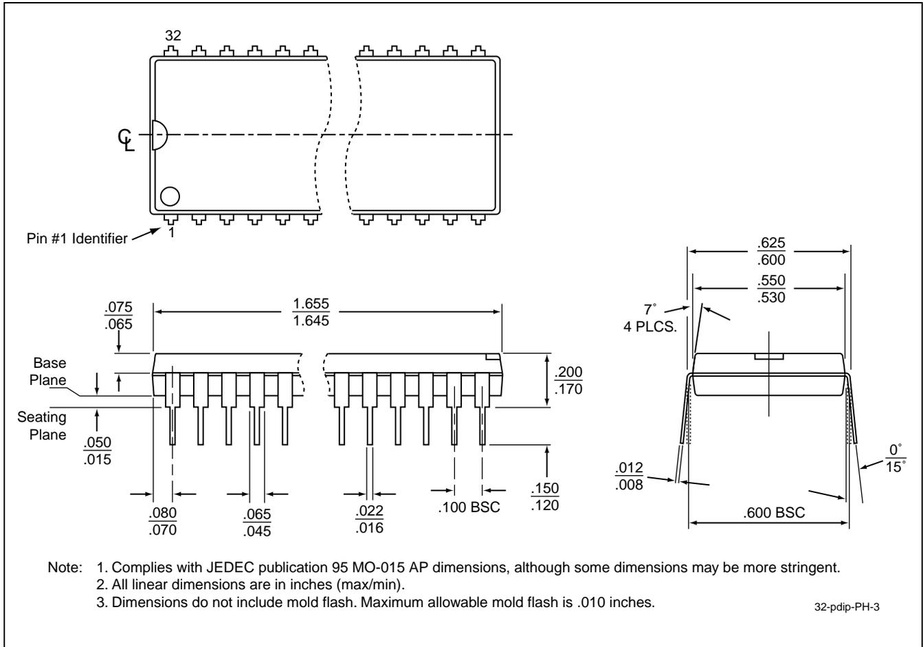
**FIGURE 19: 32-pin Plastic Dual In-line Pins (PDIP)
