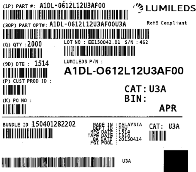
Figure 13. Example of a moisture barrier bag label.
