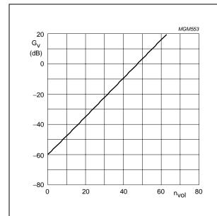
Fig.12 Volume gain as a function of volume steps.
