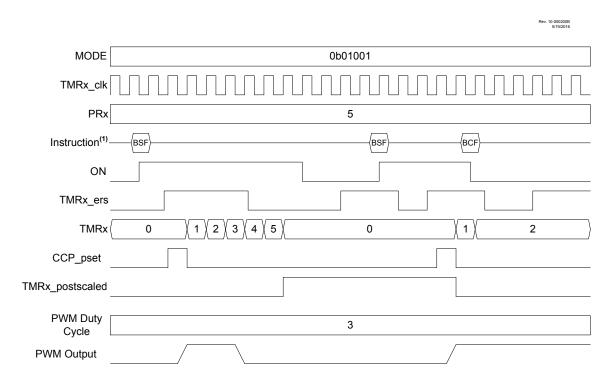
Figure 20-8. Edge-Triggered One-Shot Mode Timing Diagram (MODE = 01001)
