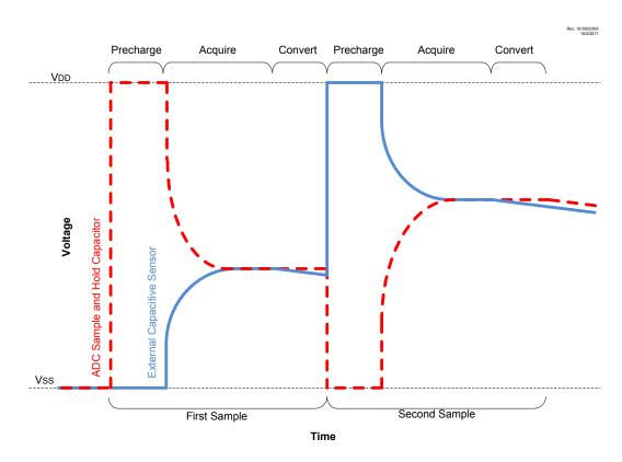
Figure 31-7. Differential CVD Measurement Waveform
