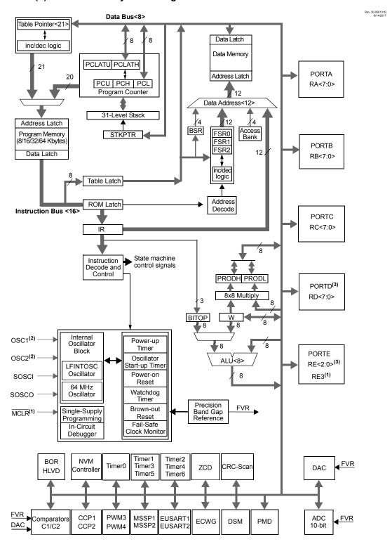
Figure 1-1. PIC18(L)F27/47K40 Family Block Diagram
