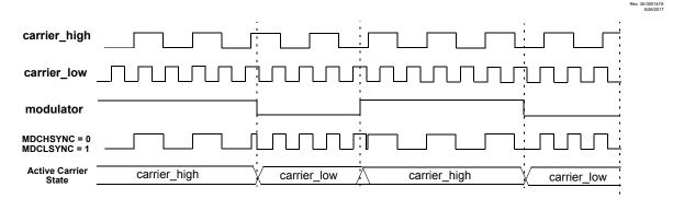
Figure 25-6. Full Synchronization (MDCHSYNC = 1, MDCLSYNC = 1)
