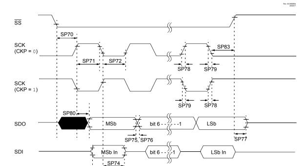
Figure 38-18. SPI Slave Mode Timing (CKE = 0)
