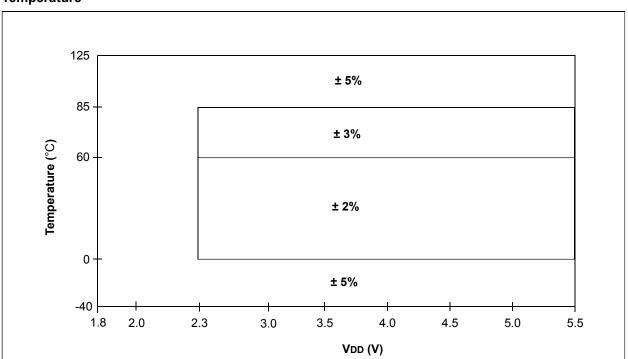
Figure 38-6. Precision Calibrated HFINTOSC Frequency Accuracy Over Device  $V_{\text{DD}}$  and Temperature
