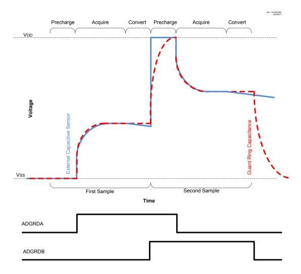
Figure 31-10. Hardware CVD Sequence Timing Diagram
