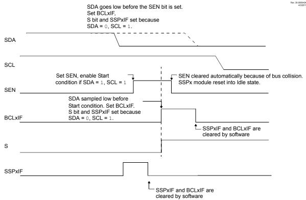
The Start condition begins with the SDA and SCL pins deasserted. When the SDA pin is sampled high, the Baud Rate Generator is loaded and counts down. If the SCL pin is sampled low while SDA is high, a bus collision occurs because it is assumed that another master is attempting to drive a data '1' during the Start condition.
