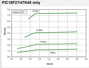
Figure 39-47.  $I_{DD}$ , HFINTOSC, Typical,
