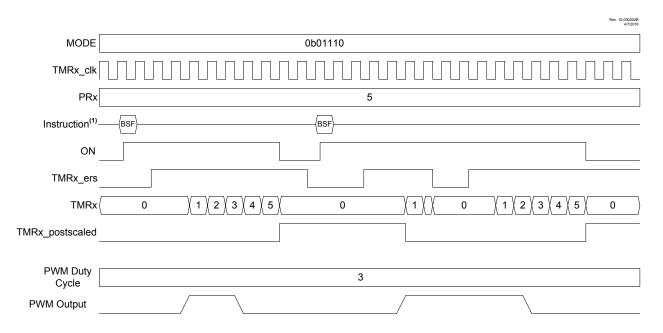
BSF and BCF represent Bit-Set File and Bit-Clear File instructions executed by the CPU to set or clear the ON bit of TxCON. CPU execution is asynchronous to the timer clock input.
