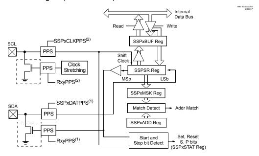
Note 1: SDA pin selections must be the same for input and output2: SCL pin selections must be the same for input and output
