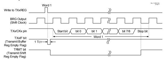
Figure 27-4. Asynchronous Transmission (Back-to-Back)
