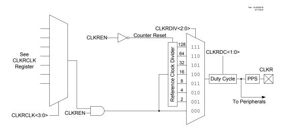
Figure 5-2. Clock Reference Timing
