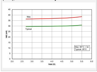
Figure 39-65. I<sub>PD</sub>, Brown-out Reset, BORV = 1, PIC18LF27/47K40 only
