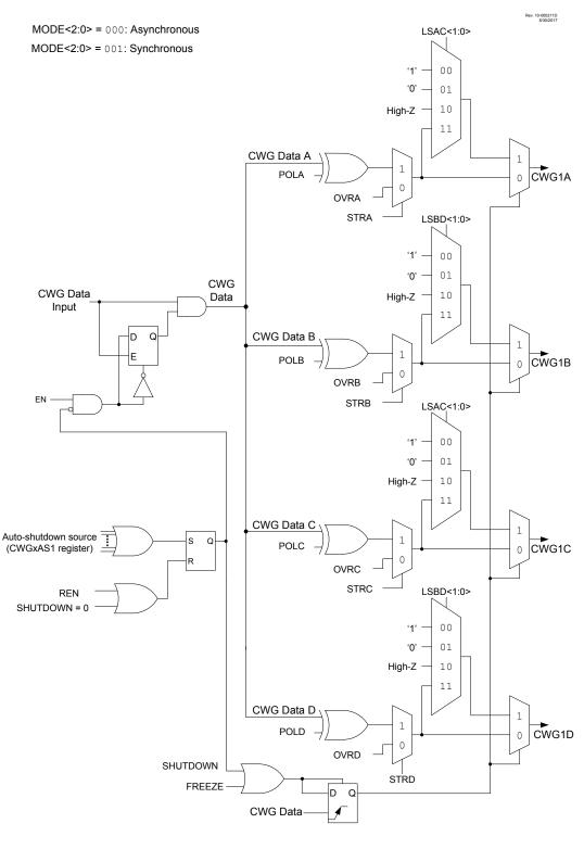
Figure 24-9. Simplified CWG Block Diagram (Output Steering Modes)
