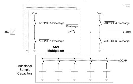
Figure 31-6. Hardware Capacitive Voltage Divider Block Diagram
