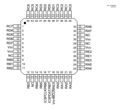
Figure 6. 44-pin QFN
