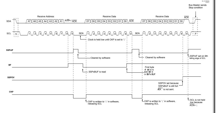
Figure 26-16. I<sup>2</sup>C Slave, 7-bit Address, Reception (SEN = 0, AHEN = 1, DHEN = 1)
