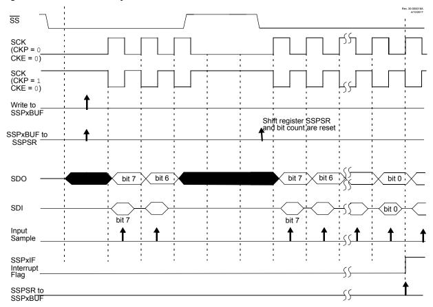
Figure 26-7. SPI Mode Waveform (Slave Mode with CKE = 0)
