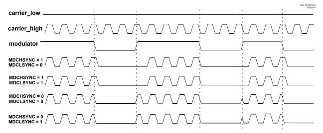
Figure 25-3. No Synchronization (MDCHSYNC = 0, MDCLSYNC = 0)
