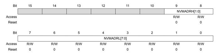
Bits 9:8 - NVMADRH[1:0] EEPROM Most Significant Address bits
