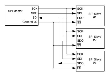
In a daisy-chain configuration, only the most recent byte on the bus is required by the slave. Setting the BOEN bit will enable writes to the SSPxBUF register, even if the previous byte has not been read. This allows the software to ignore data that may not apply to it.
