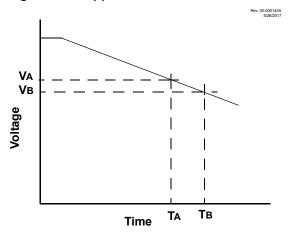
Legend: VA = HLVD trip point VB = Minimum valid device o per at ing vol tage
