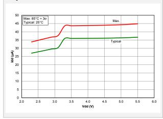
Figure 39-71. I<sub>PD</sub> Base, Low-power Sleep Mode, PIC18LF27/47K40 only
