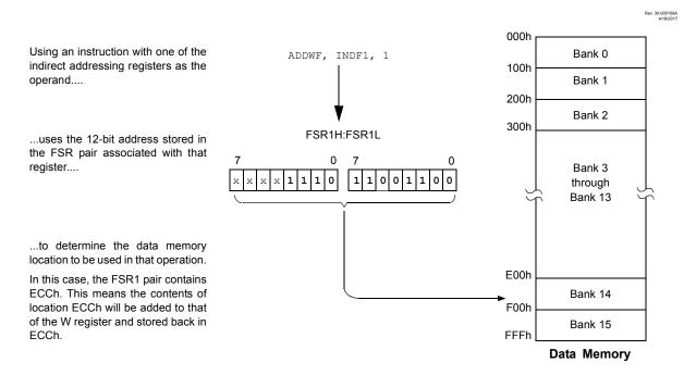
Operations on the FSRs with POSTDEC, POSTINC and PREINC affect the entire register pair; that is, rollovers of the FSRnL register from FFh to 00h carry over to the FSRnH register. On the other hand, results of these operations do not change the value of any flags in the STATUS register (e.g., Z, N, OV, etc.).
