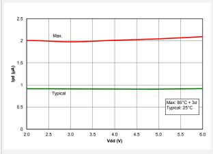
Figure 39-63. I<sub>PD</sub>, Fixed Voltage Reference (FVR), PIC18LF27/47K40 only
