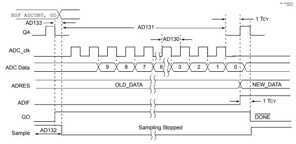
Figure 38-11. ADC Conversion Timing (ADC Clock from ADCRC)
