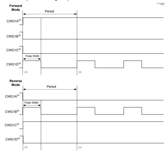
Figure 24-7. Example of Full-Bridge Output
