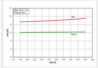
Figure 39-70. I<sub>PD</sub>, Comparator, PIC18F27/47K40 only
