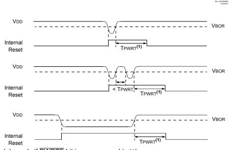
**Note:** T<sub>PWRT</sub> delay only if PWRTE bit is programmed to '0'.
