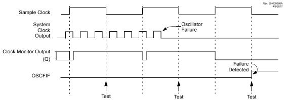
**Note:** The system clock is normally at a much higher frequency than the sample clock. The relative frequencies in this example have been chosen for clarity.
