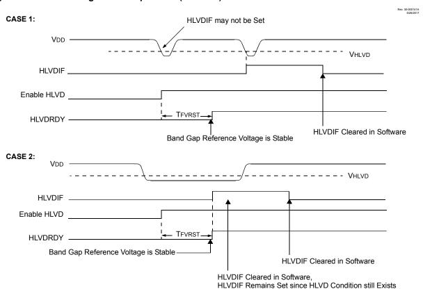
Figure 33-2. Low-Voltage Detect Operation (INTL = 1)
