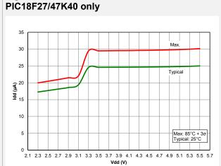
Figure 39-73. I<sub>PD</sub> Base, VREGPM = 01,
