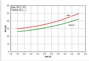
Figure 39-64. I<sub>PD</sub>, Fixed Voltage Reference (FVR), PIC18F27/47K40 only
