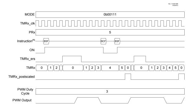
BSF and BCF represent Bit-Set File and Bit-Clear File instructions executed by the CPU to set or clear the ON bit of TxCON. CPU execution is asynchronous to the timer clock input.
