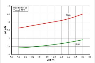
Figure 39-62. I<sub>PD</sub>, Watchdog Timer, PIC18F27/47K40 only
