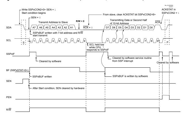
Figure 26-28. I<sup>2</sup>C Master Mode Waveform (Transmission, 7 or 10-bit Address)
