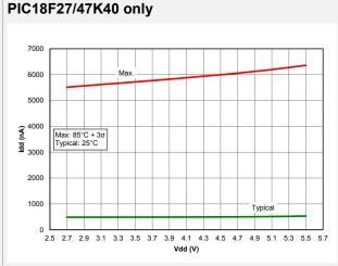
Figure 39-75. I<sub>PD</sub> Base, VREGPM = 11,
