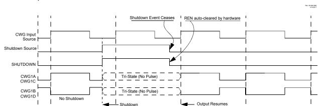
Figure 24-18. SHUTDOWN FUNCTIONALITY, AUTO-RESTART ENABLED (REN = 1, LSAC = 01, LSBD = 01)
