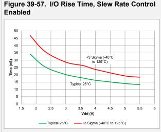
Figure 39-59. I/O Rise Time, Slew Rate Control
