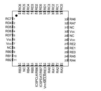
**Note:** It is recommended that the exposed bottom pad be connected to  $V_{SS}$ , however it must not be the only  $V_{SS}$  connection to the device.
