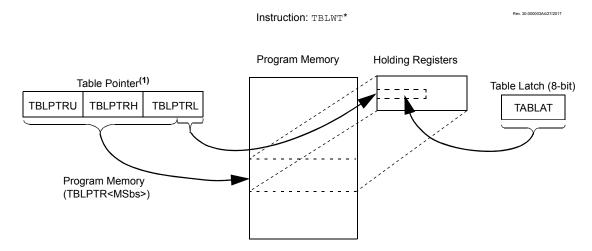
Note 1: During table writes the Table Pointer does not point directly to program memory. The LSbs of TBLPRTL actually point to an address within the write block holding registers. The MSbs of the Table Pointer determine where the write block will eventually be written.
