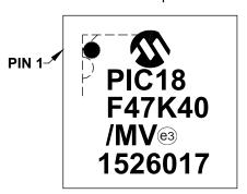
44-Lead QFN (8x8x0.9 mm)
