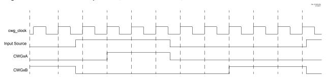
Figure 24-12. Dead-Band Operation, CWGxDBR = 0x01, CWGxDBF = 0x02
