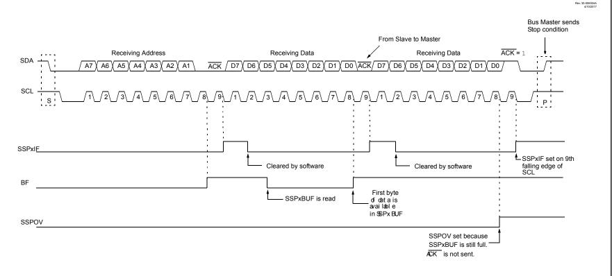
Figure 26-15. I<sup>2</sup>C Slave, 7-bit Address, Reception (SEN = 1, AHEN = 0, DHEN = 0)
