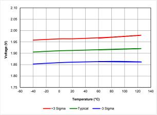
Figure 39-21. Brown-Out Reset Hysteresis, Trip Point (BORV = 11) for PIC18LF27/47K40 only
