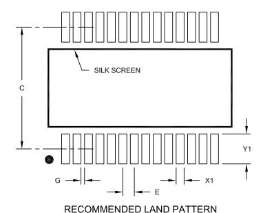
MILLIMETERS Units Dimension Limits MIN NOM MAX Contact Pitch Ε 0.65 BSC Contact Pad Spacing 7.20 С Contact Pad Width (X28) 0.45 X1 Contact Pad Length (X28) Y1 1.75 Distance Between Pads G 0.20
