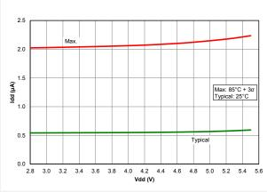
Figure 39-69. I<sub>PD</sub>, Comparator, PIC18LF27/47K40 only
