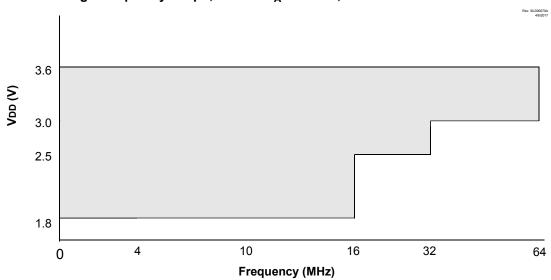
Figure 38-2. Voltage Frequency Graph, -40°C ≤ T<sub>A</sub>≤ +125°C, for PIC18LF27/47K40 Devices only
