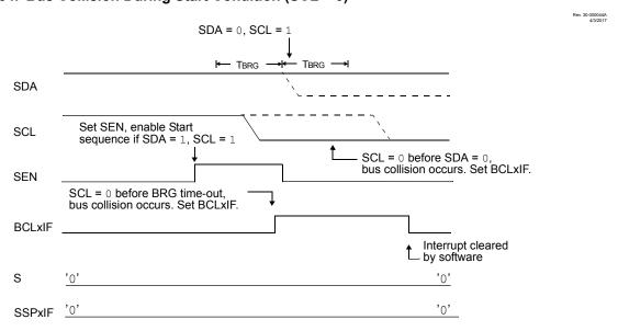
If the SDA pin is sampled low during this count, the BRG is reset and the SDA line is asserted early (Figure 26-35). If, however, a '1' is sampled on the SDA pin, the SDA pin is asserted low at the end of the
