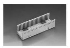
The ERmet<sup>™</sup> shroud type B is possible for a maximum of 175 contacts in 7 rows by 25 positions. The two outer rows, 2 and f are for the shielding contacts of the female connector. For this type , without multifuntion block for coding and pre-alignment, we recommend use only in combination with types A or C.
