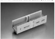
The ERmet type A vertical male connector provides 110 signal contacts and 44 ground shield contacts in 5+2 row x 25 position (3 positions used by multifunction cavity), fully loaded configuration. This connector is used in the P1 and P4 positions of a CompactPCI® backplane. With 15 different standard pin lengths to choose from, this is one of the most versatile connectors available. The connector is designed for gas tight pressfit installation.
