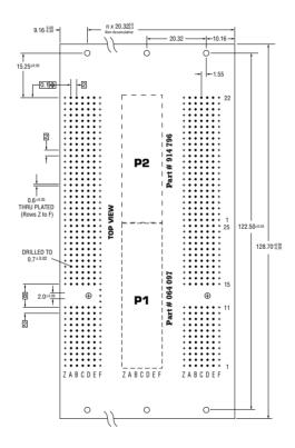
Note that the backplane is numbered in accordance with the CompactPCI® specification. The numbering on the connectors themselves is different and in accordance with the IEC 61076-4-101 standard.
