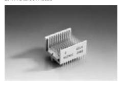
The ERmet type F vertical male connector provides 88 signal contacts and 22 ground shield contacts in a 8+2 row x 11, fully loaded configuration. With 15 different standard pin lengths to choose from, this is one of the most versatile connectors available. The connector is designed for gas tight pressft installation.
