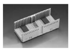
The ERmet shroud type D is possible for a maximum of 220 contacts in 10 rows by 25 positions with the length of 50 mm. The two outer rows, z and y are for the shielding contacts of the female connector. This type contains a multifunction block for coding and pre-alignment which uses 3 positions
