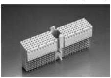
The ERmet type A female connector provides 110 contacts in a 5 row x 25 position (3 positions used by multifunction cavity), fully loaded configuration. This connector is used in the J1 and J4 positions of the CompactPCI® daughter card. The connector is designed for gas tight, pressfit installation and is provided in two different configurations: with integrated upper ground return shields and without integrated upper ground return shields. Lower ground return shields are available separately.
