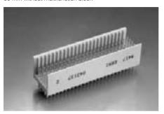
The ERmet CompactPCI type B vertical male connector provides 125 signal contacts and 50 ground shield contacts in a 5+2 row x 25, fully loaded configuration. With 15 different standard pin lengths to choose from, this is one of the most versatile connectors available. The connector is designed for gas tight pressifi installation.
