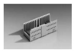
The ERmet shroud type AB is possible for a maximum of 169 contacts in 7 rows by 25 positions. The two outer rows, z and f are for the shielding contacts of the female connector. This type has pre-alignment flanges but no multifunction block for coding.
