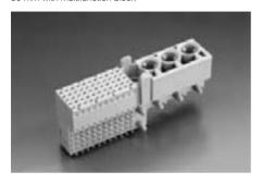
The ERmet type M female connector provides 55 contacts in a 5 row x 11 position (3 positions used by multifunction cavity), and also 3 contact positions for special power or coax contacts in a fully loaded configuration.
