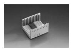
The ERmet shroud type F is possible for a maximum of 110 contacts in 10 rows by 11 positions with the length of 25 mm. The two outer rows, z and y are for the shielding contacts of the female connector.
