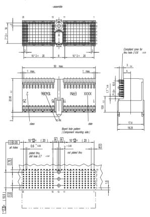
Note: The numbering on the connectors themselves is in accordance with the IEC 61076-4-101 standard. All dimensions in mm.
