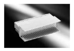
The ERmet type B right angle male connector provides 125 contacts in a 5 row x 25 position fully loaded configuration. The connector is designed for gas tight, pressfit installation and is provided in two different configurations: with integrated upper ground return shield and without integrated upper ground return shield.
