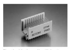
The ERmet type C vertical male connector provides 55 signal contacts and 22 ground shield contacts in 5+2 row x 11 position, fully loaded configuration. With 15 different standard pin lengths to choose from, this is one of the most versatile connectors available. The connector is designed for gas tight pressfit installation.
