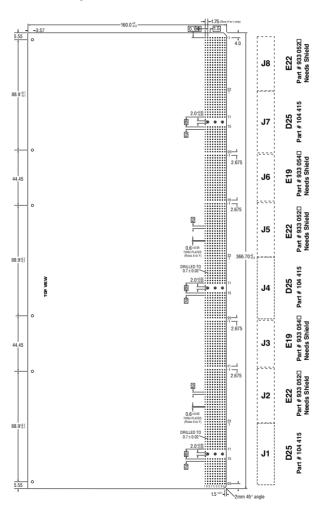
Note that the numbering scheme conforms with the Type V numbering as defined in VITA30-199x Draft 0.5 dated 9 June 1999 and is from the top down. This numbering scheme is identical to the numbering established for the connector within the IEC 61076-4-101 standard.
