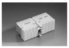
The ERmet type D female connector provides 176 signal contacts and 44 ground shield contacts in a 8 row x 25 position (3 positions used by multifunction cavity), fully loaded configuration.
