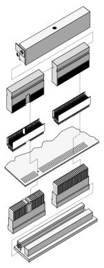
Modular press-fit tool male connector modules 5+2
