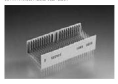
The ERmet type DE vertical male connector provides 200 signal contacts and 44 ground shield contacts in a 8+2 row x 25 position fully loaded configuration. With 15 different standard pin lengths to choose from, this is one of the most versatile connectors available. The connector is designed for gas tight pressfit installation.
