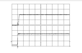
Start-up enabled by connecting V<sub>I</sub> at:  $T_{ref} = +25^{\circ}C$ ,  $I_{O} = 50$  A resistive load,  $V_{I} = 12.0$  V.
