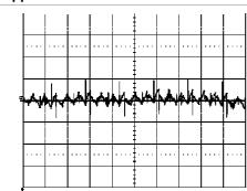
Output voltage ripple (20 mV/div.) at:  $T_{\text{ref}} = +25^{\circ}\text{C}$ ,  $I_{\text{o}} = 50$  A resistive load,  $V_{\text{i}} = 12.0$  V. Time scale: 2  $\mu\text{s}/\text{div}$ .
