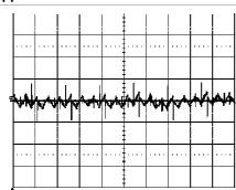
Output voltage ripple (20 mV/div.) at:  $T_{\text{ref}} = +25^{\circ}\text{C}$ ,  $I_{\text{o}} = 50$  A resistive load,  $V_{\text{i}} = 12.0$  V. Time scale: 2  $\mu\text{s}/\text{div}$ .
