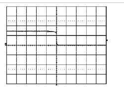
Shut-down enabled by disconnecting V<sub>I</sub> at:  $T_{\rm ref} = +25\,^{\circ}\text{C}$ , I<sub>O</sub> = 50 A resistive load, V<sub>I</sub> = 12.0 V.
