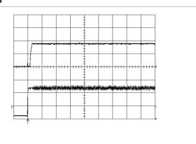
Start-up enabled by connecting V<sub>I</sub> at:  $T_{ref} = +25^{\circ}C$ ,  $I_{O} = 50$  A resistive load,  $V_{I} = 12.0$  V.
