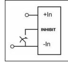
The products are equipped with a Inhibit control function referenced to the primary negative input connection (- In), positive logic. The INHIBIT function allows the regulator to be turned on/off by an external device like a semiconductor or mechanical switch.
