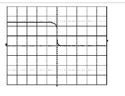
Shut-down enabled by disconnecting V<sub>I</sub> at:  $T_{\rm ref} = +25\,^{\circ}\text{C}$ , I<sub>O</sub> = 50 A resistive load, V<sub>I</sub> = 12.0 V.
