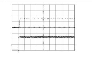
Start-up enabled by connecting V<sub>I</sub> at:  $T_{ref} = +25^{\circ}C$ ,  $I_{O} = 50$  A resistive load,  $V_{I} = 12.0$  V.
