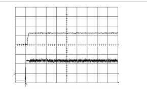
Start-up enabled by connecting V<sub>I</sub> at:  $T_{ref} = +25^{\circ}C$ ,  $I_{O} = 50$  A resistive load,  $V_{I} = 12.0$  V.
