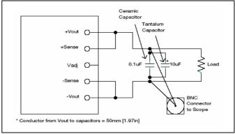
Output ripple and noise test setup
