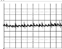
Output voltage ripple (20 mV/div.) at:  $T_{\rm ref} = +25^{\circ}C$ ,  $I_{0} = 50$  A resistive load,  $V_{1} = 12.0$  V. Time scale: 2  $\mu$ s/div.
