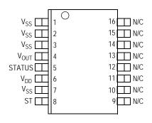
16-Pin SOIC Package N/C pins are recommended to be left FLOATING
