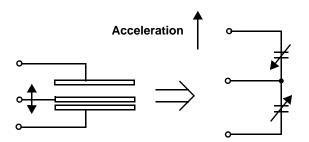
Figure 3. Transducer Physical Model
