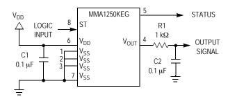
Figure 5. SOIC Accelerometer with Recommended Connection Diagram
