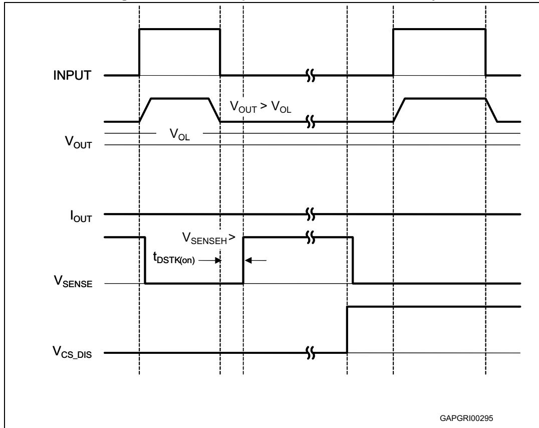
Figure 15. Short to V<sub>CC</sub>
