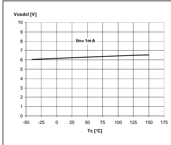
**Figure 30. Low level CS\_DIS voltage**
