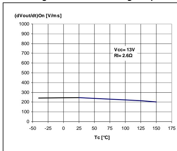
**Figure 28. Turn-off voltage slope**
