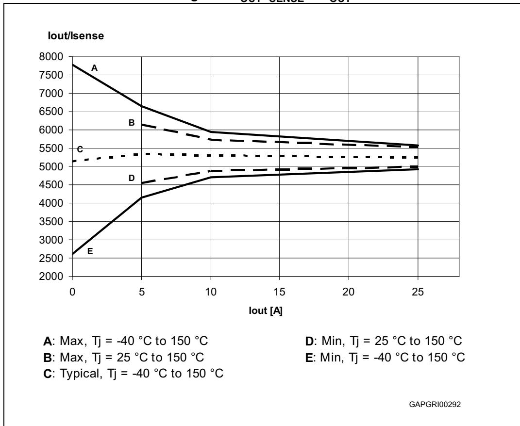
**Figure 7. Maximum current sense ratio drift vs load current**
