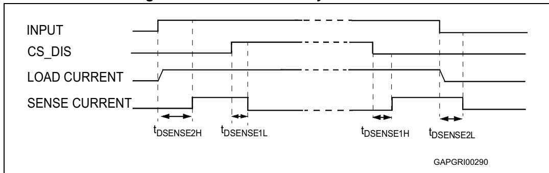
**Figure 5. Open-load off-state delay timing**
