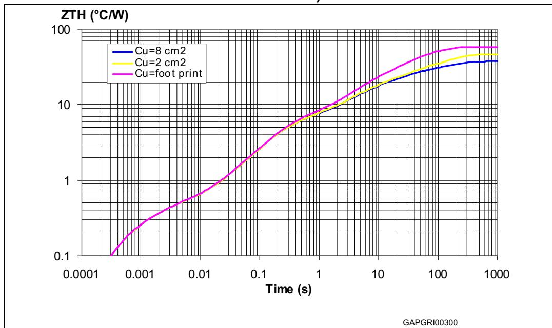
**Figure 38. Thermal fitting model of a double channel HSD in PowerSSO-36<sup>(1)</sup>**
