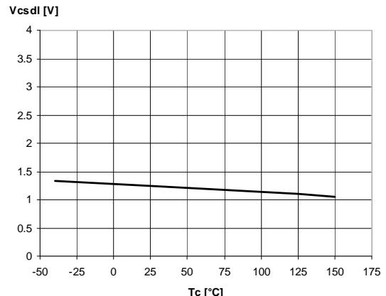
**Figure 31. High level CS\_DIS voltage**
