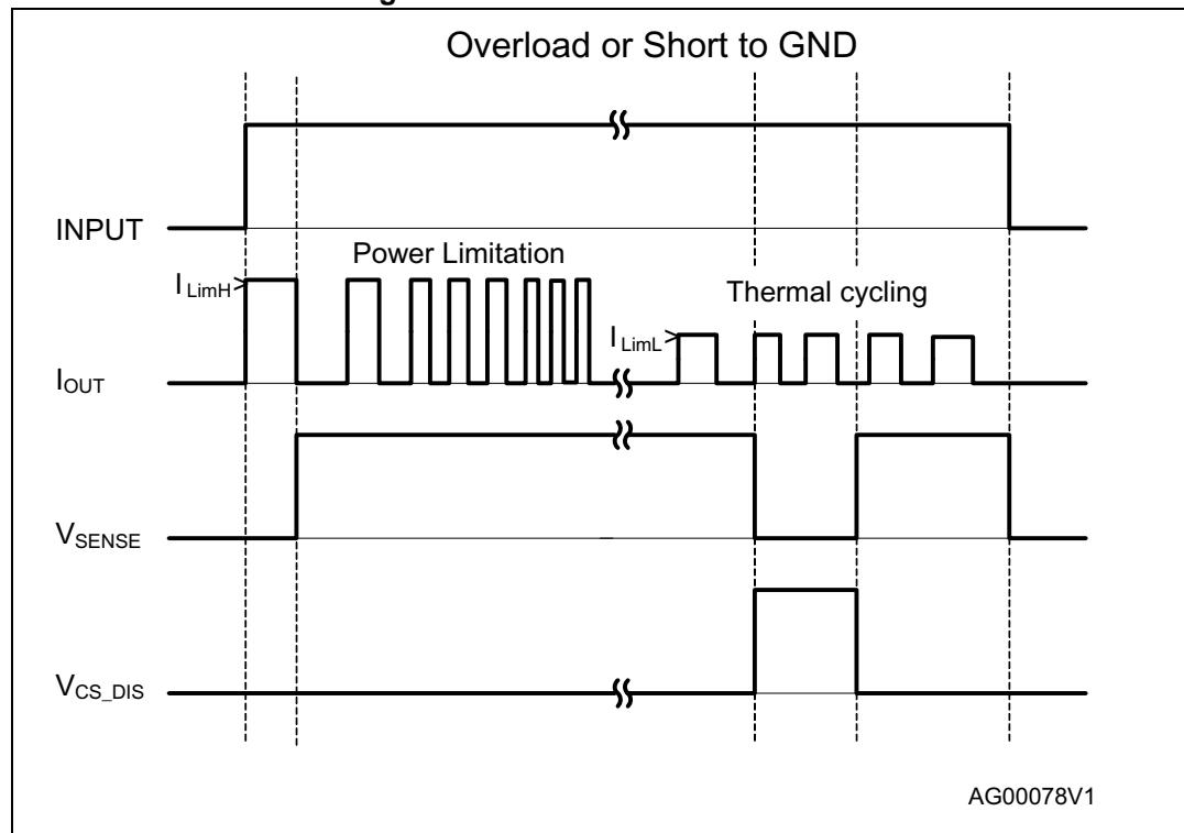
**Figure 13. Intermittent overload**
