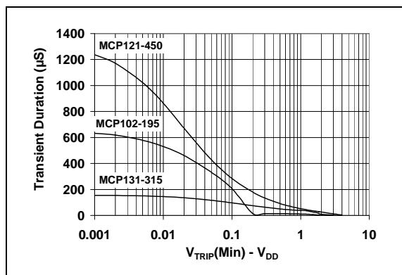
**FIGURE 2-32:** Transient Duration vs.  $V_{TRIP}(\text{min}) - V_{DD}$ .
