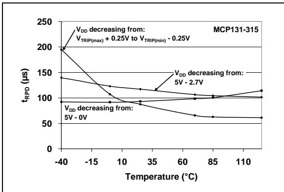
**FIGURE 2-24:**  $t_{RPD}$  vs. Temperature
