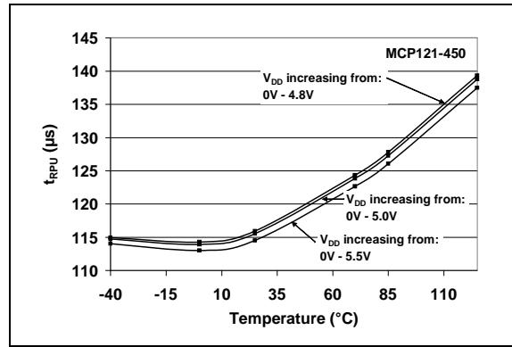
**FIGURE 2-28:**  $t_{RPU}$  vs. Temperature
