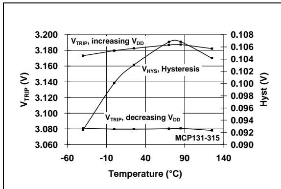
**FIGURE 2-14:**  $V_{TRIP}$  vs. Temperature vs. Hysteresis (**MCP131-315**).
