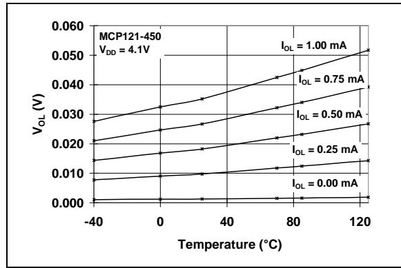
**FIGURE 2-21:**  $V_{OL}$  vs. Temperature
