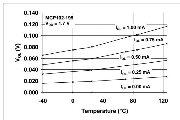
**FIGURE 2-19:**  $V_{OL}$  vs. Temperature
