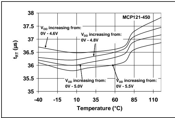
**FIGURE 2-25:**  $t_{RPD}$  vs. Temperature
