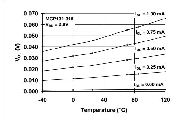
**FIGURE 2-20:**  $V_{OL}$  vs. Temperature
