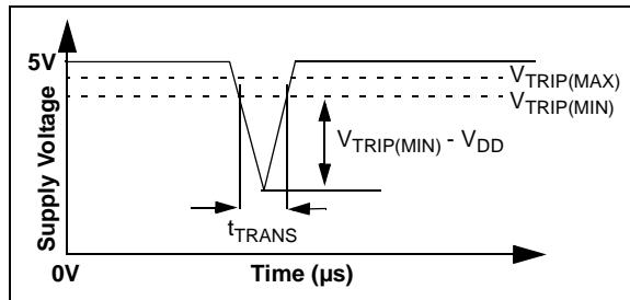
**FIGURE 4-3:** Example of Typical Transient Duration Waveform.
