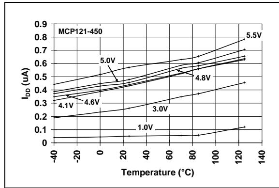
**FIGURE 2-3:**  $I_{DD}$  vs. Temperature
