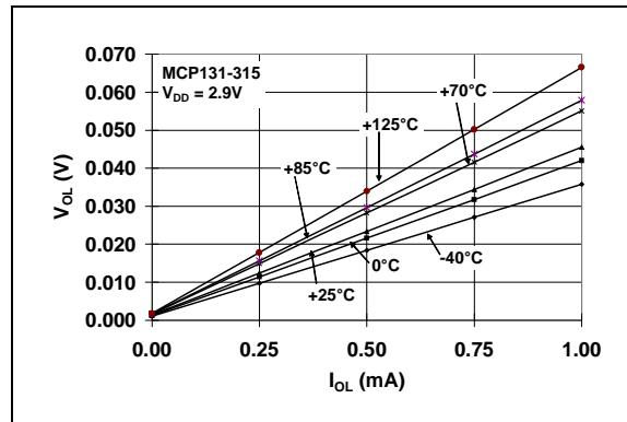
**FIGURE 2-17:**  $V_{OL}$  vs.  $I_{OL}$  (**MCP131-315** @  $V_{DD} = 2.9V$ ).
