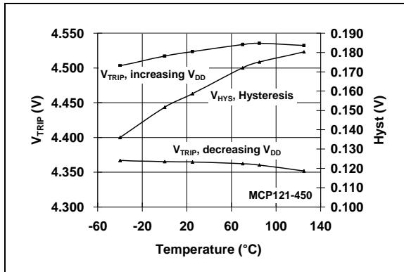
**FIGURE 2-15:**  $V_{TRIP}$  vs. Temperature vs. Hysteresis (**MCP121-450**).
