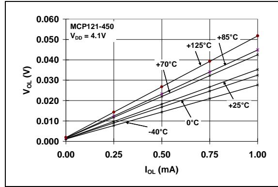
**FIGURE 2-18:**  $V_{OL}$  vs.  $I_{OL}$  (**MCP121-450** @  $V_{DD} = 4.1V$ ).
