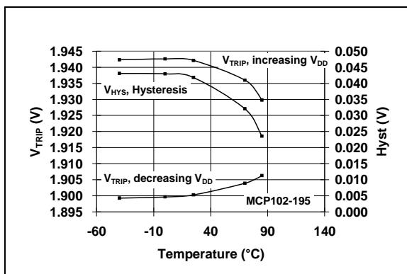
**FIGURE 2-13:**  $V_{TRIP}$  vs. Temperature vs. Hysteresis (**MCP102-195**).
