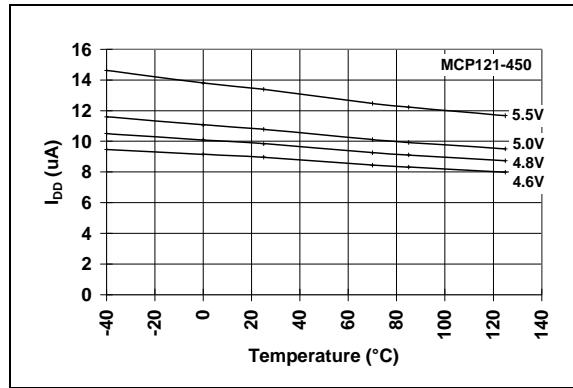
**FIGURE 2-6:**  $I_{DD}$  vs. Temperature
