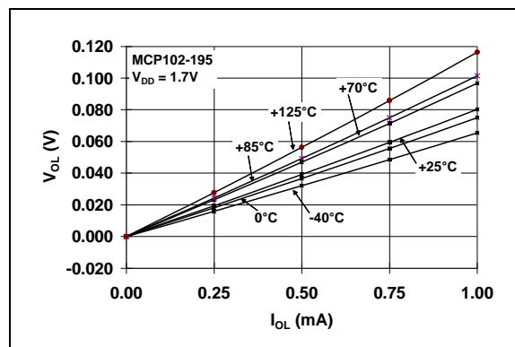
**FIGURE 2-16:**  $V_{OL}$  vs.  $I_{OL}$  (**MCP102-195** @  $V_{DD} = 1.7V$ ).
