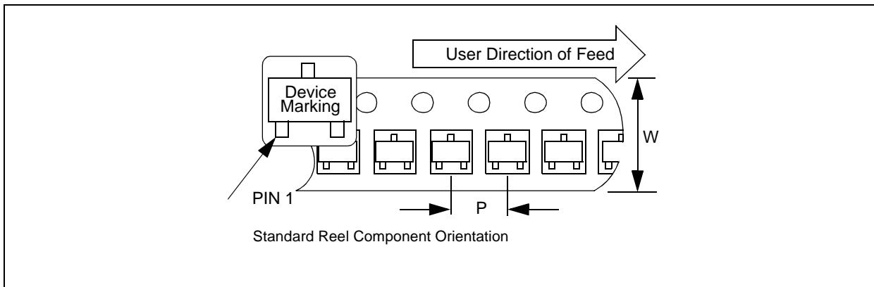
**FIGURE 5-3: TO-92 DEVICE TAPE AND REEL SPECIFICATIONS**
