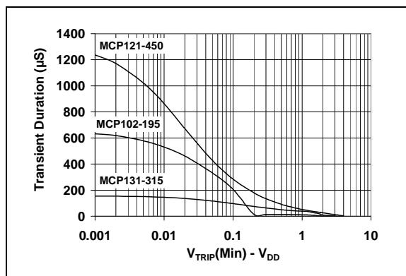
**FIGURE 2-32:** Transient Duration vs.  $V_{TRIP}(min) - V_{DD}$ .
