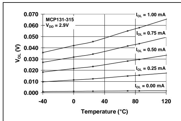
**FIGURE 2-20:**  $V_{OL}$  vs. Temperature
