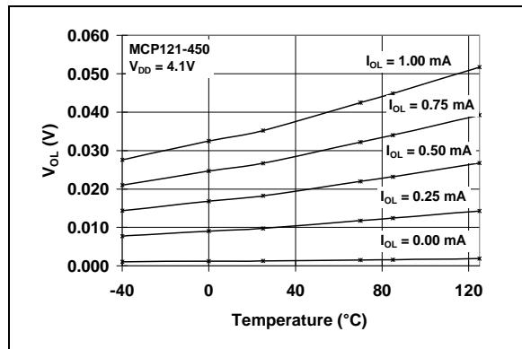
**FIGURE 2-21:**  $V_{OL}$  vs. Temperature
