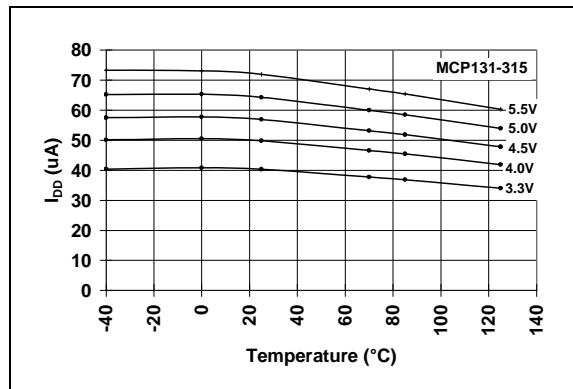
**FIGURE 2-5:**  $I_{DD}$  vs. Temperature
