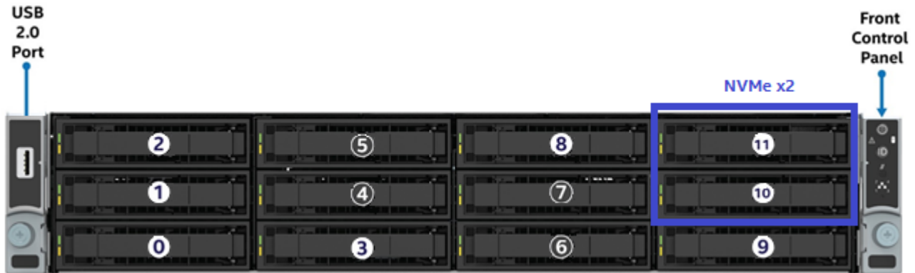
Figure 42. 3.5" drive bay, 12 drive configuration
