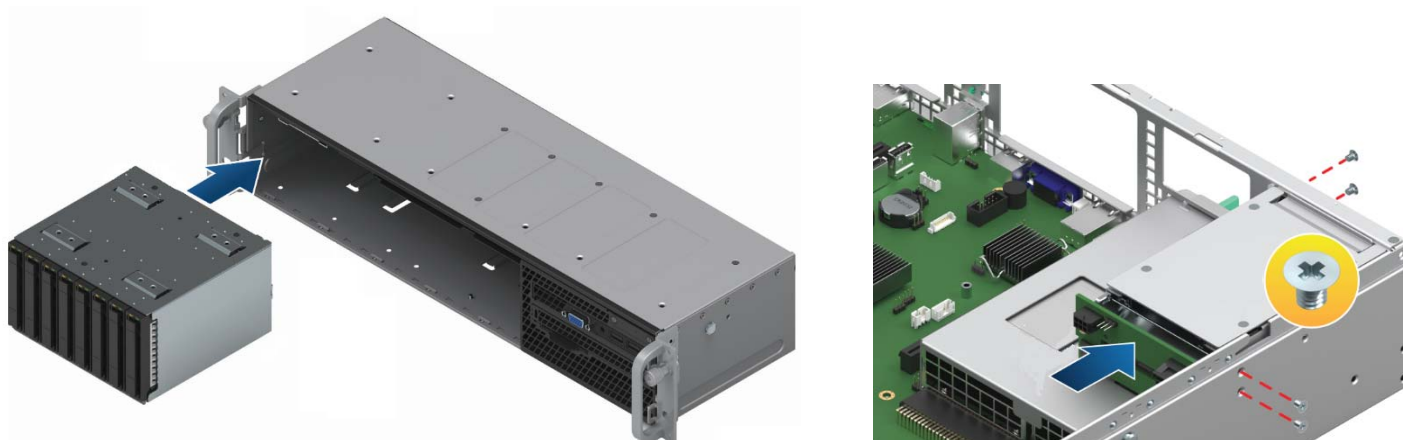
Figure 48. 2.5" drive bay module placement options
