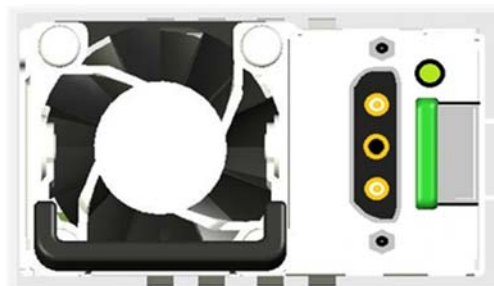
DC Power Cable Connectors
