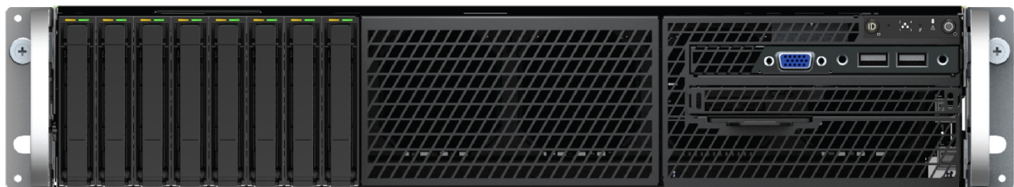
Figure 12. 2.5" x 8 front drive bay configuration – R2208WFxxxx
