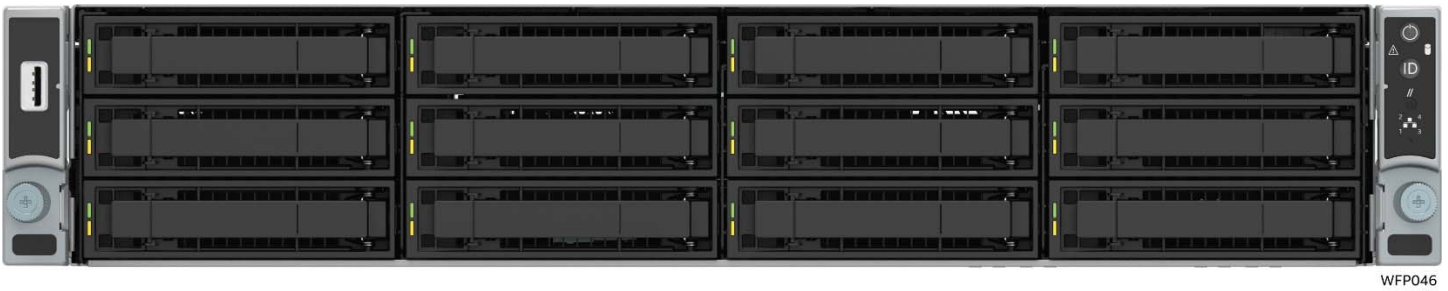
Figure 11. 3.5" x 12 front drive bay configuration – R2312WFxxxx
