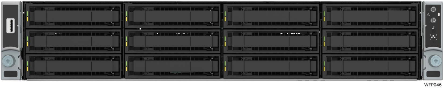
Figure 11. 3.5" x 12 front drive bay configuration – R2312WFxxxx
