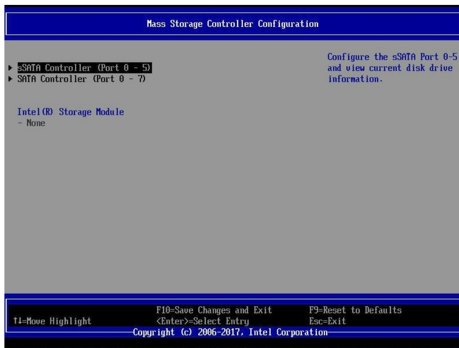
Figure 61. BIOS setup Mass Storage Controller Configuration screen
