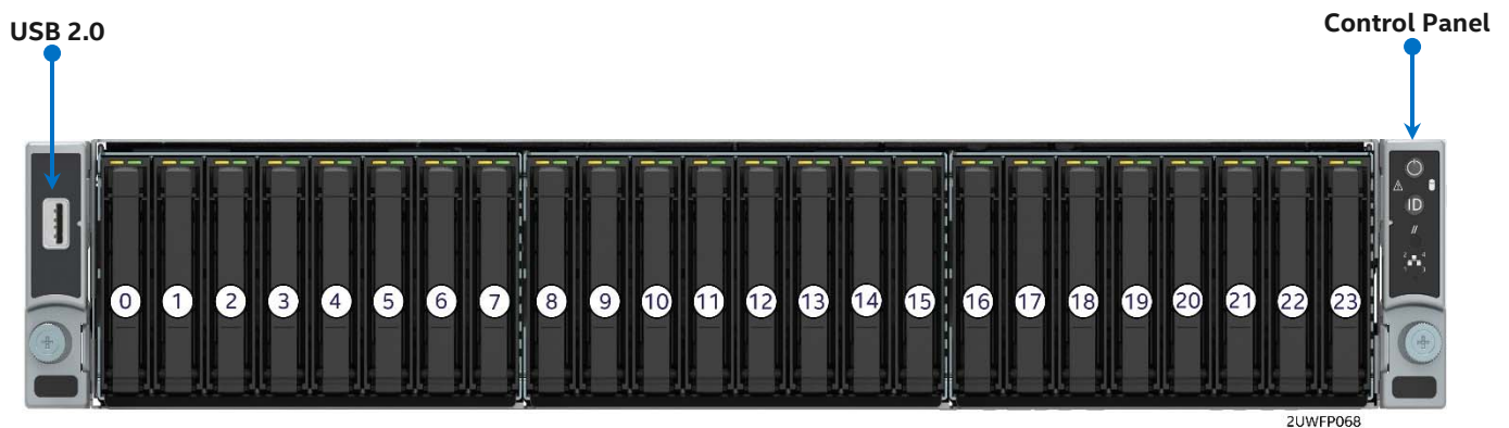
Figure 40. 2.5" front mount drive bay, 24 drive (R2224WFxxx) configuration
