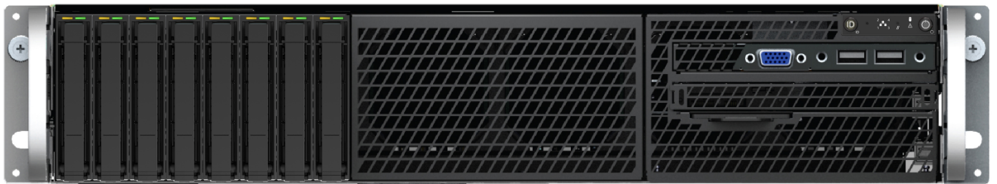
Figure 12. 2.5" x 8 front drive bay configuration – R2208WFxxxx
