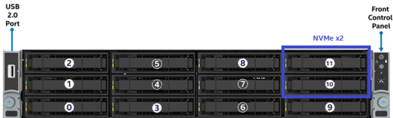
Figure 42. 3.5" drive bay, 12 drive configuration
