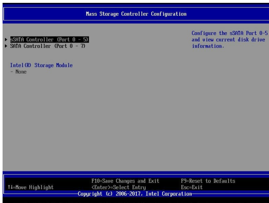
Figure 61. BIOS setup Mass Storage Controller Configuration screen
