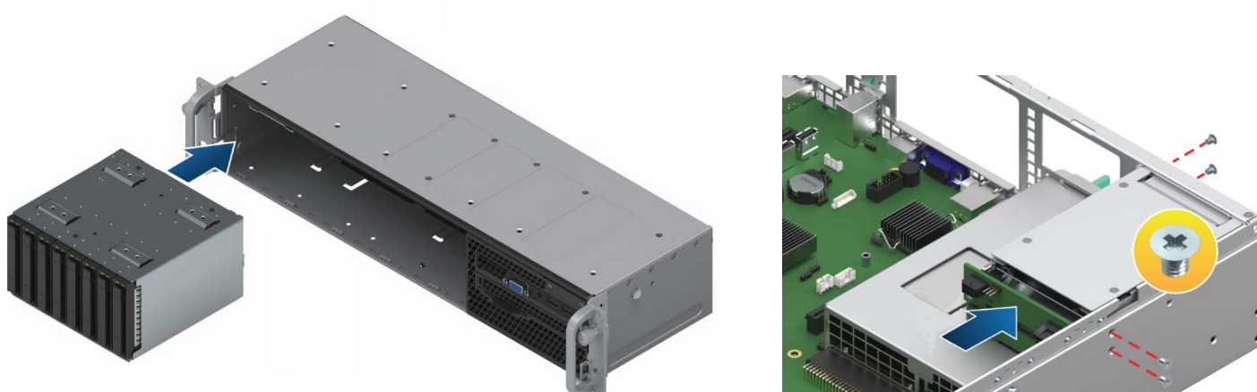
Figure 48. 2.5" drive bay module placement options
