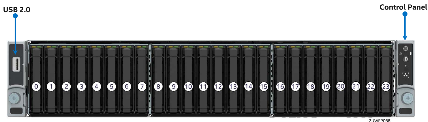
Figure 40. 2.5" front mount drive bay, 24 drive (R2224WFxxx) configuration
