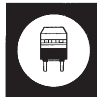
Stand-Off Lugs Minimize Solder-Creepage
