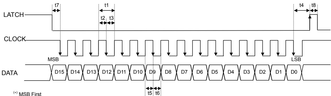
Note.) Set CLOCK in High to prevent incorrect operation during a standby period.
