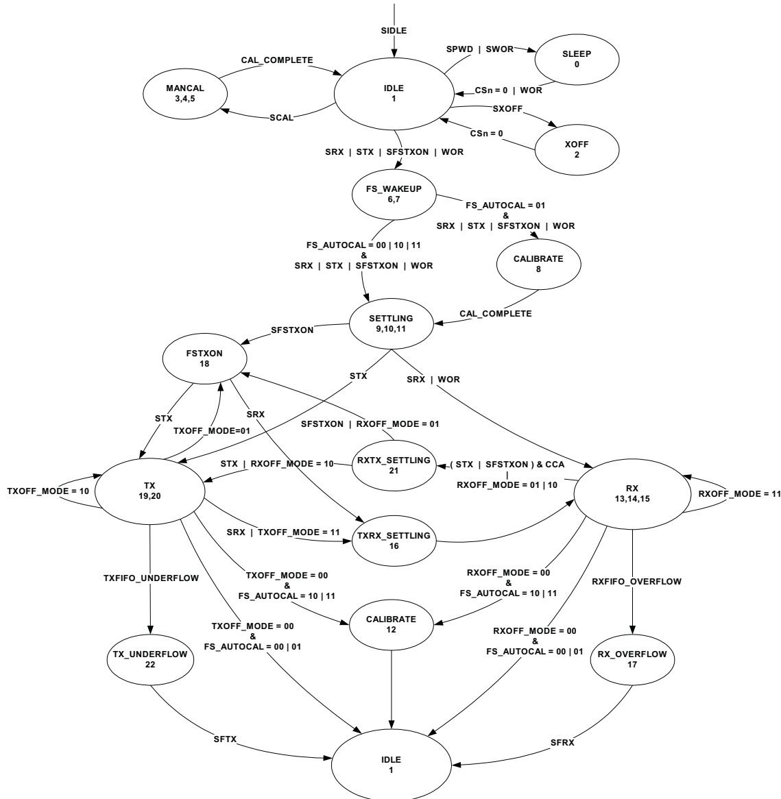
Figure 3-15. Complete Radio-Control State Diagram
