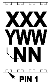
14-Lead SOIC (150 mil) (MCP6H74)
