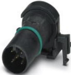
Sensor/actuator flush-type connector, plug, 5-pos., A-coded, with angled solder connection, only contact insert
