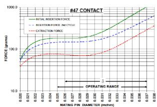
racteristics above were derived using 30 microinch gold plate and polished steel gauge pins having a bullet-shaped tip.
