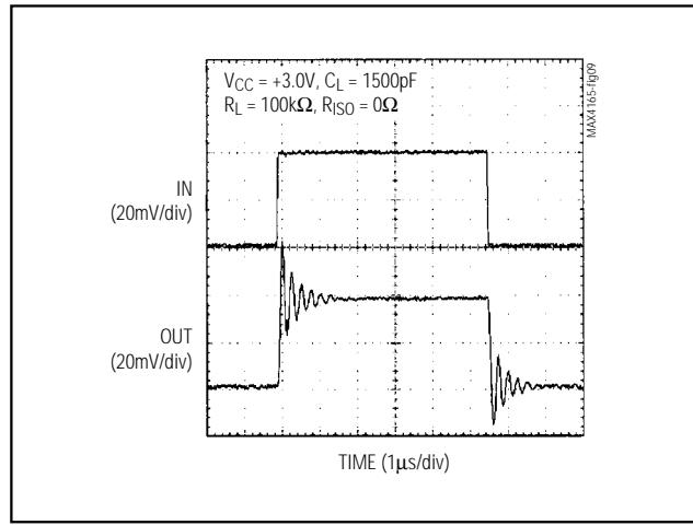
Figure 9. Small-Signal Transient Response with Excessive Capacitive Load
