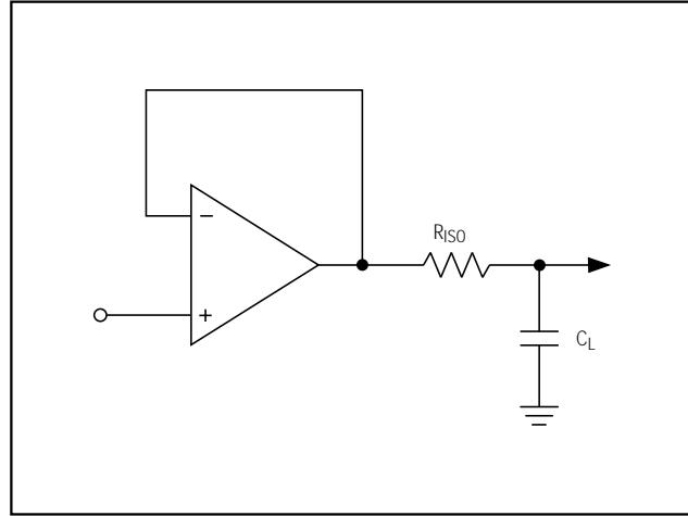
Figure 11. Capacitive-Load-Driving Circuit
