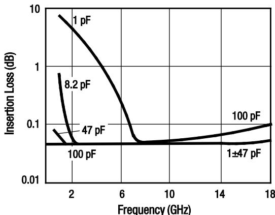
**Figure 1. Typical Insertion Loss vs Frequency
