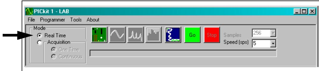
In Real-time mode, data conversions are performed immediately and transmitted to the PC. The data is displayed on a real-time strip chart.
