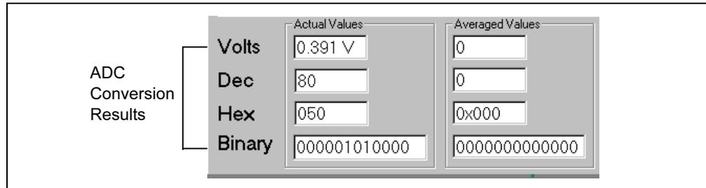
A second set of values provides the ability to observe the effects of averaging (Figure 2-7). When Averaging is selected, the Rolling Average mode is enabled. The display is updated after every conversion based on the average of the last  $n$  conversions where  $n$  = counts.
