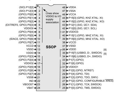
Figure 2-3. 48-pin SSOP Part Pinout
