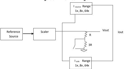
Figure 8-7. DAC Block Diagram
