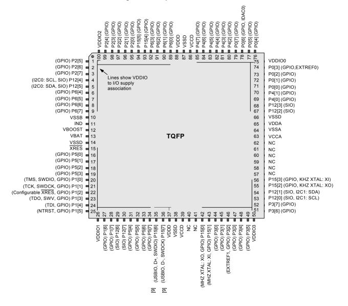
Figure 2-6. 100-pin TQFP Part Pinout
