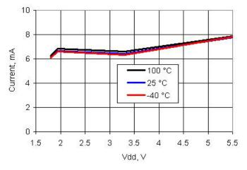
Figure 11-2. Active Mode Current vs Temperature and F<sub>CPU</sub>,  $V_{DD}^{-} = 3.3 \text{ V}$
