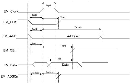
Figure 11-55. Synchronous Read Cycle Timing
