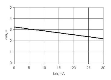
Figure 11-23. USBIO Output Low Voltage and Current, GPIO Mode
