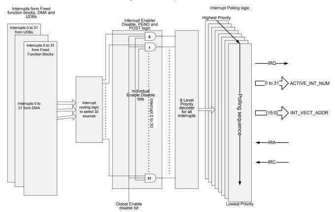
Figure 4-3. Interrupt Structure
