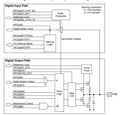
Figure 6-10. SIO Input/Output Block Diagram
