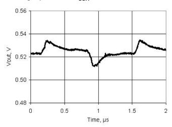
Figure 11-51. VDAC Voltage Noise, 1 V Mode, High speed mode,  $V_{\rm DDA}$  = 5 V
