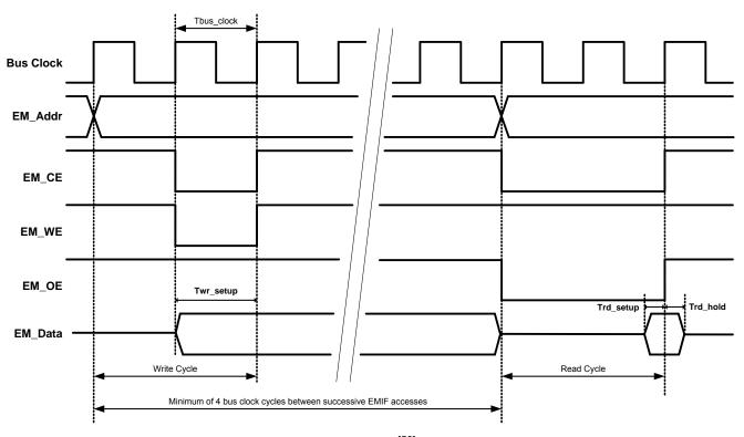
Table 11-53. Asynchronous Write and Read Timing Specifications<sup>[56]</sup>
