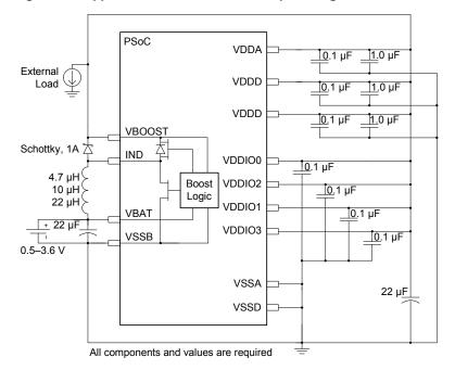
Figure 6-6. Application of Boost Converter powering PSoC device
