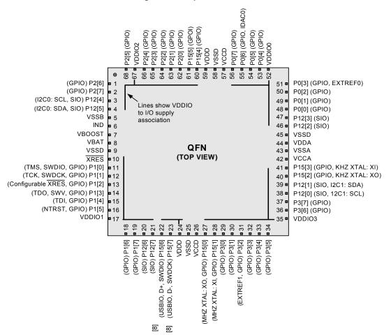
Figure 2-5. 68-pin QFN Part Pinout<sup>[7]</sup>
