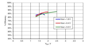
Figure 11-12. Efficiency vs  $V_{BAT}$ ,  $L_{BOOST}$  = 10  $\mu H^{[35]}$
