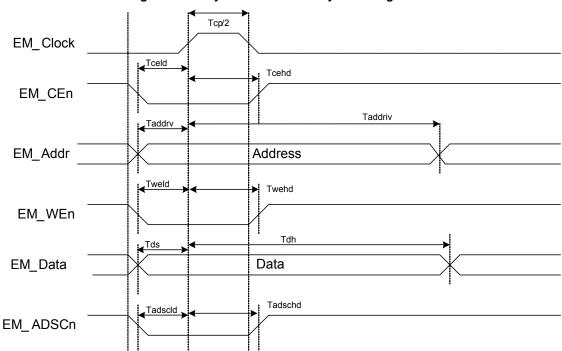
Figure 11-56. Synchronous Write Cycle Timing
