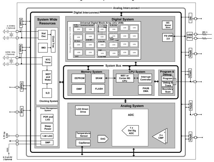
Figure 1-1. Simplified Block Diagram
