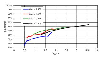
Figure 11-13. Efficiency vs  $V_{BAT}$ ,  $L_{BOOST}$  = 22  $\mu H$  [35]
