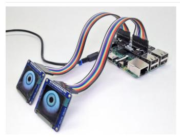
Here's a probable layout for a non-portable installation. **Straight header pins** have been soldered to the bonnet board and the displays, projecting "up" and "back," respectively. Two 11-pin **female-to-female** ribbon cables then join everything.
