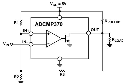
Figure 22. Inverting ADCMP370 Comparator Configuration with Hysteresis
