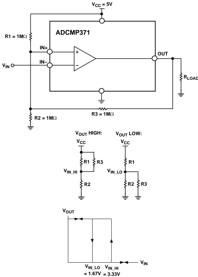
Figure 20. Inverting ADCMP371 Comparator Configuration with Hysteresis
