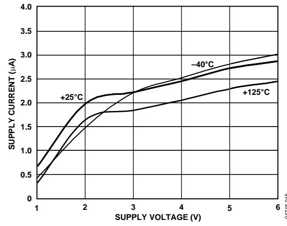
Figure 9. Supply Current vs. Supply Voltage (Output High)
