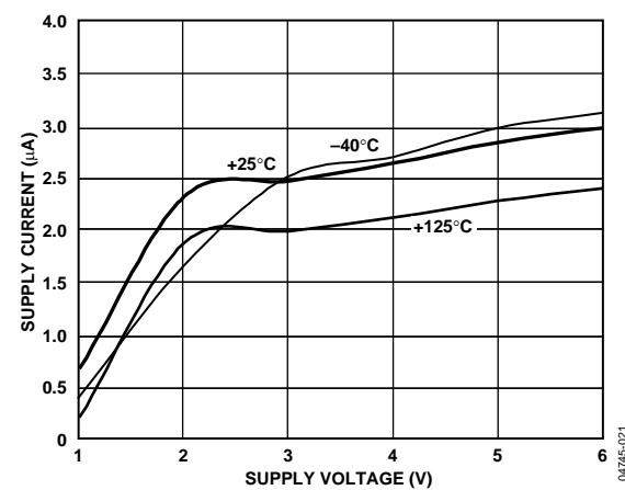
Figure 8. Supply Current vs. Supply Voltage (Output Low)
