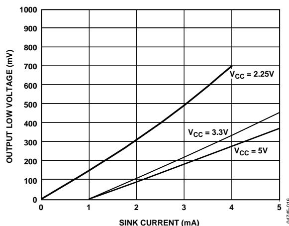
Figure 10. Output Low Voltage vs. Sink Current
