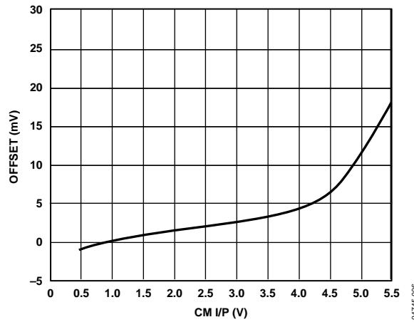
Figure 4. Input Offset vs. Common-Mode Input Voltage
