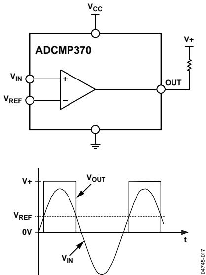
Figure 18. Basic Comparator and Input and Output Signals
