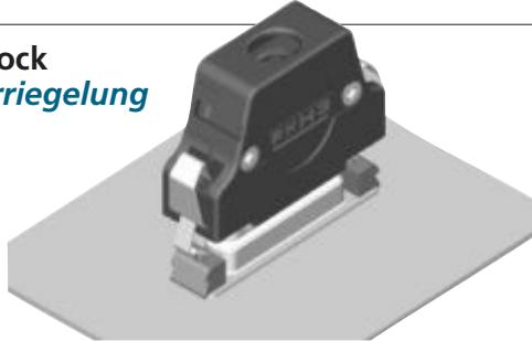
The latch lock can be inserted without a tool. It consists of two latch inserts F-GK1/5, two locking screws FSGK1/5 and both locking springs FFB1/5. With the use of a locking screw, the locking insert is mounted to the shell of the mating connector. The locking springs are fixed to the hood. This type of locking system is suitable for hoods in the FPHGR, FKH, FPHF and FPHRS-3 and 4 series.
