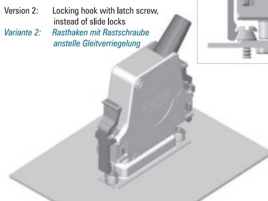
Metal hood FMK3 with two locking hooks. The two latch screws, e. g. F62M091S245 are mounted on the front panel. They act as opposite locking elements. The maximum front panel thickness is 6,0 mm (0.236").
