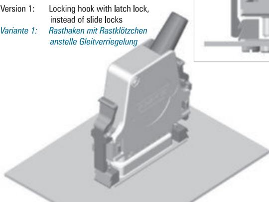
Metal hood FMK3 with two locking hooks FRH1/5. The two latch locks F-GK1/5 are fixed by two rear side mounted locking screws FSGK1/5 on the front panel. They act as opposite locking elements. The maximum front panel thickness is 2,5 mm (0.098").
