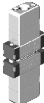
Cable to cable connection of two waterproof D-Sub connectors with FMH hoods by using locking screws, threaded spacers, washers and front seal.
