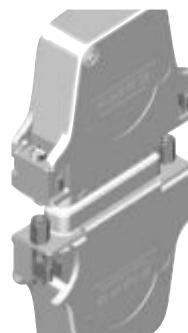
Cable to cable connection of two D-Sub connectors with FMK hoods by using locking screws and female standoff nuts F1066.
