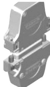
Cable to cable connection of two D-Sub connectors with FMK and FMH hoods by using locking screws, threaded block inserts and female screw locks F-GSCH1/5.
