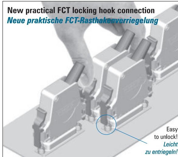
The new locking hook connection, as an alternative to slide locking, facilitates the use of this type of locking device even with our metal hoods. This swiftly released connector locking device is thus ideal for applications in areas which require EMI / EMC secure mating. The advantage: The simplest of mounting, as the locking hook can be snapped in place within a few seconds once hood assembly has been completed.
