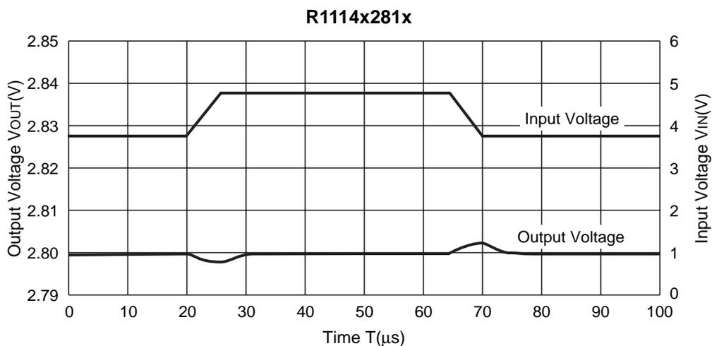
11) Load Transient Response ( $t_r=t_f=0.5\mu s$ ,  $C_{IN}=\text{Ceramic } 1.0\mu F$ )
