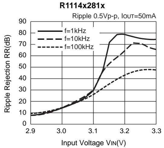
9) Ripple Rejection vs. Frequency (C<sub>IN</sub>=none)
