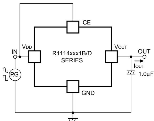
Fig.3 Ripple Rejection, Line Transient Response Test Circuit
