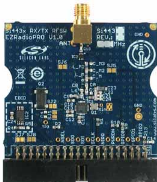
Figure 17. Single-Ended TX and RX Testcard
