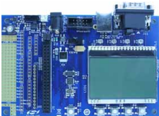
Figure 1. MSC-DBSB8 Software Development Board (SDB)
