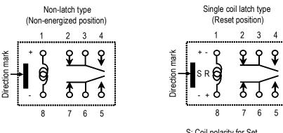
S: Coil polarity for Set R: Coil polarity for Reset
