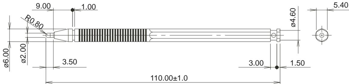
Note: The dimensional tolerance is  $\pm 0.5\text{mm}$  unless otherwise specified. Not to scale.
