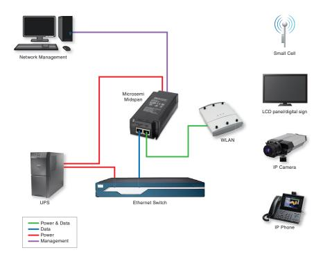
Microsemi single and multiport midspans are an economical and easy way to power popular devices such as WLAN access points, IP video phones, IP security cameras, security access devices, thin clients and printers over new or existing Ethernet infrastructure.
